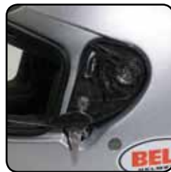
Shield crack position #2
