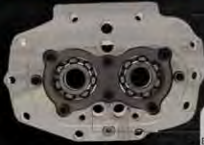
STOCK PLASTIC CAGED DOOR BEARINGS, RETAINED WITH .060" THICK INTERNAL SNAP RINGS
