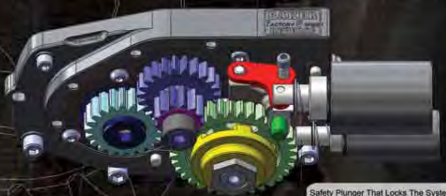
Safety Plunger That Locks The System Out Of Reverse While The Bike Is Not In Neutral & The Toggle Switch Is Off
