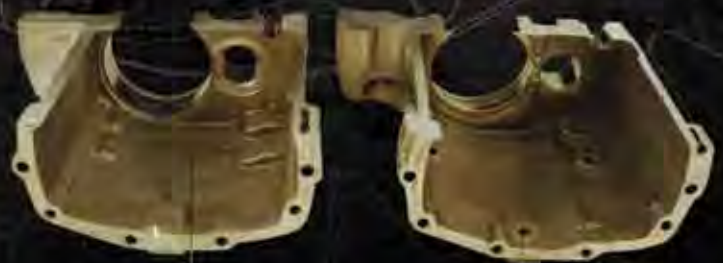
5 CASTED IN PADS TO ELIMINATE ANY POTENTIAL LEAK THROUGH THE TRANSMISSION STUDS
