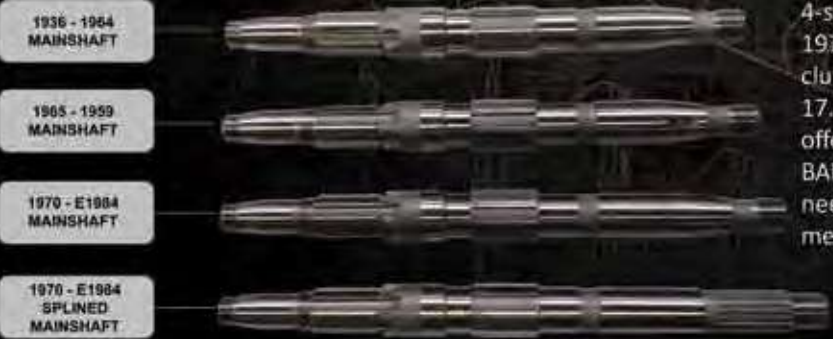
ALL MAINSHAFTS HAVE CAGED NEEDLE BEARING LANDINGS
