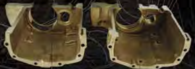
5 CASTED IN PADS TO ELIMINATE ANY POTENTIAL LEAK THROUGH THE TRANSMISSION STUDS
