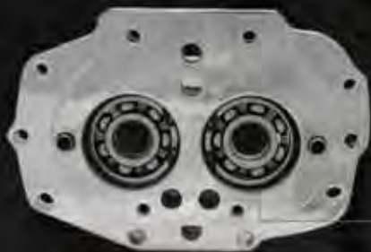
STOCK PLASTIC CAGED DOOR BEARINGS
