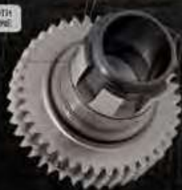
BAKER MAIN DRIVE GEAR WITH 6 TOOTH SPLINE SPLINE DIAMETER IS 1.75" ABOUT A 1/4" LARGER THAN A STOCK MAIN DRIVE GEAR
