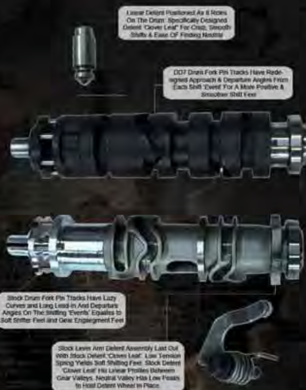
DD7 vs Stock Shift Drum
