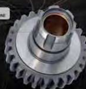
STOCK 4-SPEED MAIN DRIVE GEAR WITH 5 TOOTH SPLINE SPLINE DIAMETER IS 1.50" ABOUT A 1/4" DIFFERENCE FROM THE BAKER GEAR
