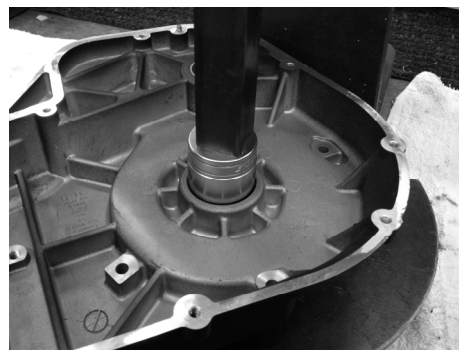
BEARING REMOVAL, FIGURE 2
