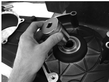
BEARING INSTALLATION, FIGURE 3
