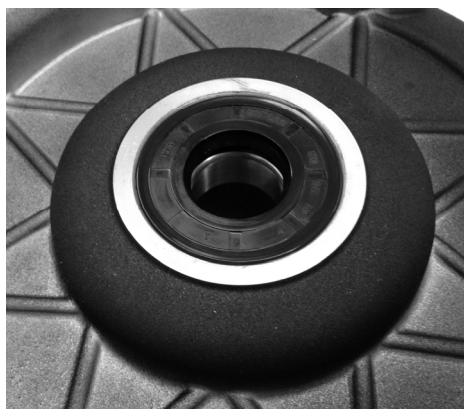
SEAL INSTALLED, FIGURE 5
