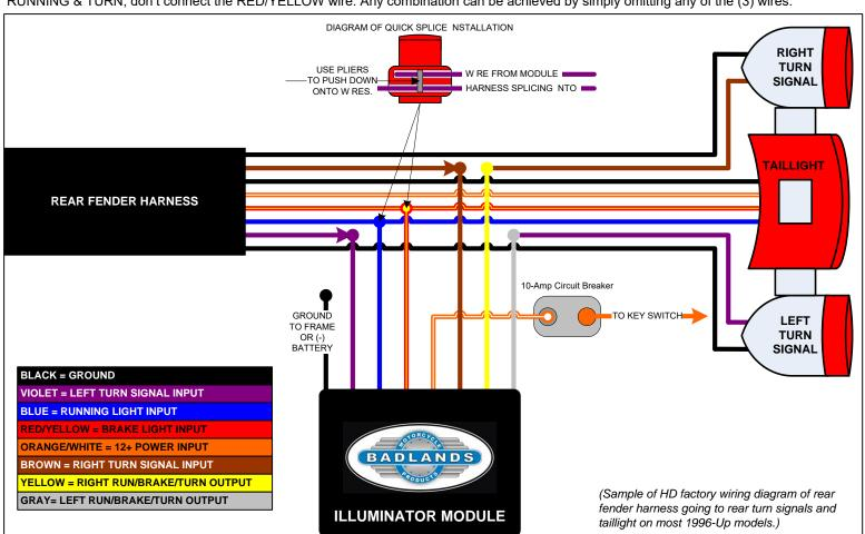
The wire colors in the drawing will not be the same on all models but do match most 1996-up factory HD motorcycles. If you have a pre-1996 model be sure to consult your bikes service manual for exact wiring diagrams and color descriptions to achieve proper installation.
