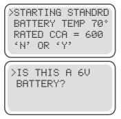
Confirm that the inputs are correct. Press 'Y' if they are correct. The test will start. Press 'N' to re-enter temp, battery rating and battery type.
