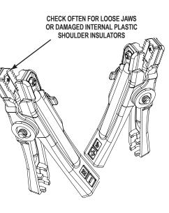
connection, the threaded stud connects to the smaller gauge wire that reads the voltage, and the load pad ring connects to the larger conducting wire that draws the load in each test. Damaged clamps or loose wires will affect the readings. Keep clamps clean and in good repair.
