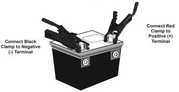
Use the side terminal feature on the clamp to connect battery side terminals. When testing dual post batteries always check the post to which the system is attached.
