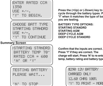
cycle through the battery types. Press 'Y' when it matches the type of battery
