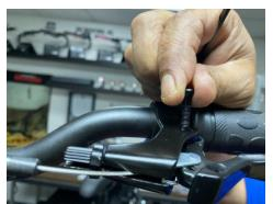
Locate the brake lever bolt on the brake perch. Use the 4mm Allen on brake lever bolt to loosen. Remove the bolt, the spring, the lever, the washer, and the nut. Keep the bolt and nut
