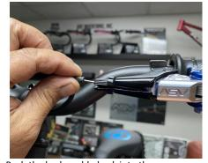
Push the brake cable back into the perch and tighten the brake cable adjustor all the way.
