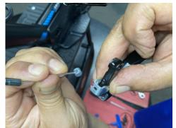
Remove the brake cable anchor from the brake lever
