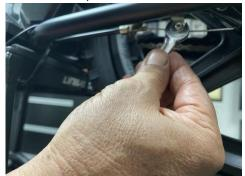
Locate the brake cable arm underneath the swingarm on the brake side about 3 inches from the axle. Use the 10mm wrench to loosen the brake cable nut.
