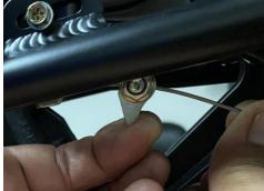
To secure the rear, pull the brake cable arm frontward until it stops. While holding, pull the brake cable rearwards just enough to remove the slack. Then tighten the nut.
