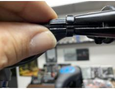
Locate the brake cable adjuster on the brake perch. Use your fingers to loosen the adjuster and line up the openings so that the cable can be removed.
