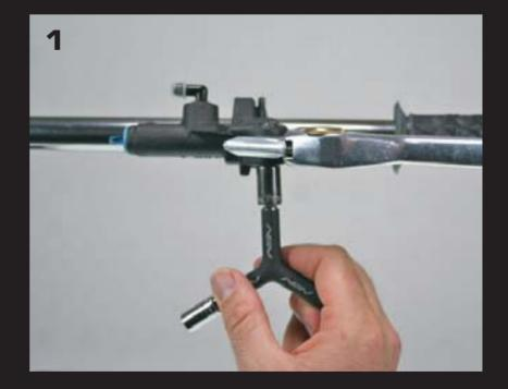
10mm wrench or socket to remove the locknut attached to the main pivot bolt that holds the lever. (Photo 1)
