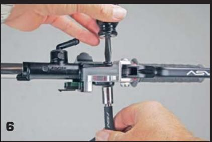
IMPORTANT: Be sure to adjust the reach of your lever to fit your hand properly, yet still allow enough movement to properly engage your clutch.
