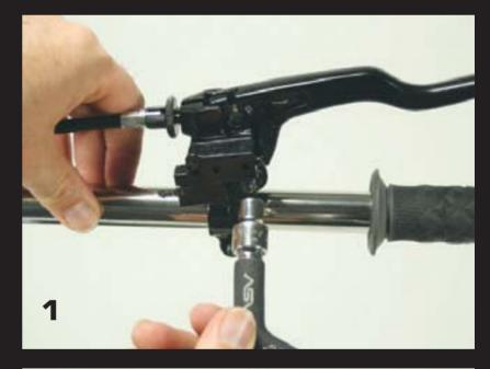
Pull the cable away from the perch to expose the inner-wire. You will need to pull very hard to do this. (No damage can occur as you will be simply engaging your clutch slightly while doing this) Guide the inner wire through the adjuster and perch. Then remove the cable barrel from the clutch lever to completely detach the cable from your clutch lever.
