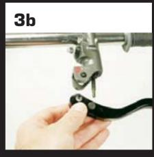
reach adjust knob until it is completely out of the barrel attached to the stock lever. (Photo 3a) Now the lever can be completely removed from the master cylinder. (Photo 3b)
