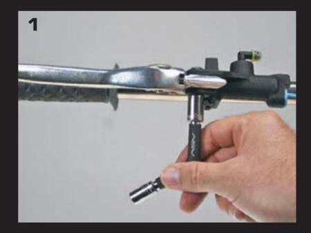
10mm wrench or socket to remove the locknut attached to the main pivot bolt that holds the lever. (Photo 1)
