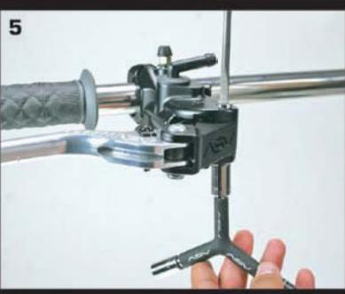
locknut as it can cause binding of the lever and master cylinder. Maximum torque on locknut should be five (5) foot-lbs. or sixty (60) inch-lbs.
