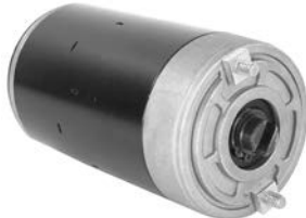
SAB0123 For Monarch Pump Motor 12-Volt; CCW; LESTER 10762; PIC 106-318; 3 Inch Permanent Magnet Motor Ball Bearing DE Frame 1/4 Inch Slot in Shaft 14-20 Thru Bolts 6mm Output Stud 6mm Ground Stud The Ground Stud Does Not Have to Be Connected for the Unit to Operate REPL.: REFERENCE NUMBER 14785, 17208, 2590100, -12, 262174, 50501, 56539, 8110, 82195, 8301, M2590112, M4100; WESTERN MOTORS W-8031, W-8031-D
