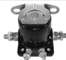
SFD6006 Solenoid, Remote 12-Volt; 4-Terminal;
