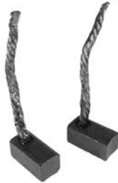
SPL9107 Brush Set For Prestolite Starters PIC 5460-6061; 6.4mm T x 6.3mm W x 12mm L Used on Small Prestolite Motors REPL.: PRESTOLITE 42-32, ESQ12S, Q12S
