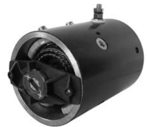
LWAA001 For Boom Lift Arms on Trucks, Latent Paving Box Equipment, Etc. Pump Motor 24-Volt; CW; PIC 160-934; Special Slot Shaft w/Bushing at the Drive End Slot Thru Bolts are at 3 O'Clock and 9 O'Clock REPL.: WAPSA 9130450044; WESTERN MOTORS W-8872
