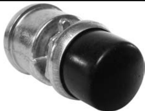
SSW2814 Push Button Switch PIC 9900-9014; 2-Screw Terminals ON-OFF (Normally OFF) Switch 2 Threaded Bosses with Screws for Wire Connections Plastic Button O-Ring Seal in Mounting Stem Protective Cap and Face Nut Assembly REPL.: COLE HERSEE 90030-01, 90030BP, 9095, 9244, 9244-02, 9245; DELCO D907
