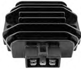
AYA6035 Voltage Regulator / Rectifier For Yamaha Scooters
