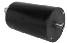
SAB0167 For Western Plows Snow Plow Motor 12-Volt; CW; LESTER 10770; PIC 160-710; 3 Inch Diameter Permanent Magnet Motor Shaft Diameter .625 Inch .20 Inch Slot in Shaft REPL.: BOSCH F-000-MM0-804; FISHER 48543; WESTERN MOTORS W-6804; WESTERN PLOW 27753
