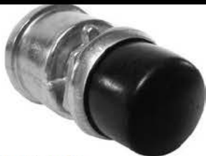
SSW2814 Push Button Switch PIC 9900-9014; 2-Screw Terminals ON-OFF (Normally OFF) Switch 2 Threaded Bosses with Screws for Wire Connections Plastic Button O-Ring Seal in Mounting Stem Protective Cap and Face Nut Assembly REPL.: DELCO D907
