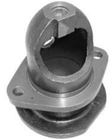
SDR2084 D/E Housing PIC 5640-1012; Lester 4093; 2 Inch Distance From Base of Housing (Where It Meets The Field Case) To Mounting Surface REPL.: DELCO 1962387
