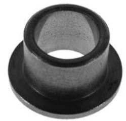
STC7103 Bushing, C/E For Tecumseh Starters PIC 6-12710; ID 9.53mm OD 12.7mm OAL 9.65mm 17.8mm Flange
