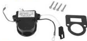
PL105-207 Voltage Regulator, OEM 12-Volt; B-Circuit; For Motorola Alternators Set Point 14.2 Volts; Activation Ignition; B-Circuit; Negative Ground; Terminal ID Red - Trio (+) Black - Ground Green - Field Yellow - IGN; Short Keyhole Case Style; Used on Motorola Alternators REPL.: MOTOROLA 5-207, 8RG2009A; PRESTOLITE 105-207
