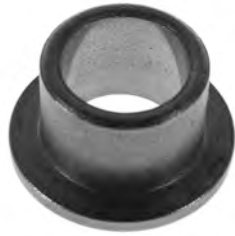
STC7103 Bushings, C/E For Tecumseh Starters PIC 6-12710; ID 9.53mm OD 12.7mm OAL 9.65mm 17.8mm Flange Used on Tecumseh Starters
