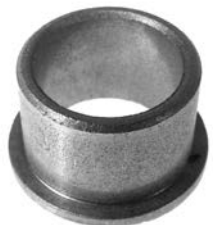
STC7102 Bushing, D/E For Tecumseh Starters PIC 6-15080; ID 12.7mm OD 15.93mm OAL 11.43mm 19.0mm Flange
