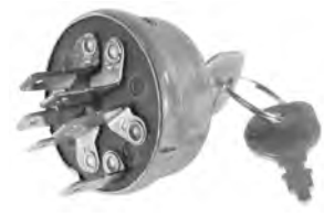
SSW2826 Key Switch Lawn & Garden Applications PIC 9900-9026; 4-Position 6-Terminal 5/8 Mounting Stem Used on Murray REPL.: BRIGGS & STRATTON 5411H; MURRAY 092377MA, 792377, 92377
