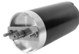
SAB0159 For Warn Winch Winch Motor 12-Volt; Bi-Directional; LESTER 10785; PIC 106-655; 3 Inch Motor 3/8 Inch Drive Tang Terminals are 6mm x 1.0 REPL.: WARN WINCH 21592, -594; WESTERN MOTORS W-8092, W-8092B, -2D
