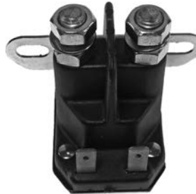
SSE6016 Solenoid, Remote 12-Volt; 4-Terminal; PIC 6699-116;
