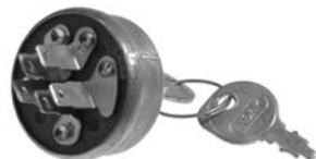
SSW2817 Key Switch Lawn & Garden Applications PIC 9900-9017; 3-Position 5-Terminal 5/8 Mounting Stem Can Use SSW9200 Wiring Harness Used on Honda H1011, H1011H, H1011HK1, H2013SA, H2013SAC, H2013HK1SAC John Deere JD321 Commercial Walk Behind Mowers, 111 Series (Below 1200) Toro Sand Pro Aerators, Greensmaster 3000G, and Reelmaster 216 REPL.: AYP / ROPER 3621R, 365402, 3L5402, 4406R, -LR, STD365402; BOBCAT 48032B; HONDA 35100-772-003; HUSQVARNA 532365402; JOHN DEERE AM102551; LAWN-BOY 23-0660, 700172, 741308; MTD 725-0267, 725-0267A, 925-0267, 925-0267B; MURRAY 21064, 421064; TORO 23-0660; TROY BILT 1908112, 925-0267B
