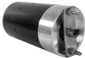
SAB0125 For Superwinch Winches and Tarp Covers Winch/Tarp Motor 12-Volt; Bi-Directional; LESTER 10763; PIC 106-317; 2-Post 4.3mm Flat Tang Shaft Shaft Diameter .52 Inch 1/4-20 Thru Bolts REPL.: REFERENCE NUMBER 1102, -110, -307, -646, B01-006A; SUPERWINCH 1110; WESTERN MOTORS W-8023
