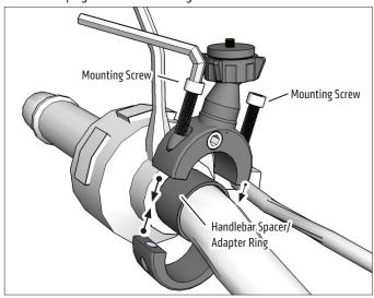
Adjust camera position as desired. Tighten adjustment ring to secure position.
