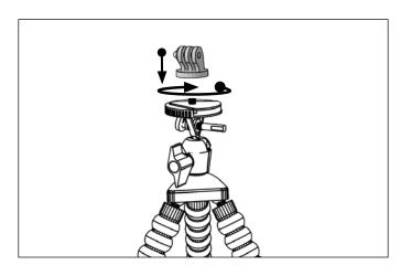
2 Unscrew lateral screw and insert GoPro HERO (sold separately) to the adapter. Re-insert lateral screw.
