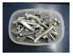
This is a small collection of levers that I have broken or found on the ground in the pits. This is one of the motivating factors to make the ARC folding lever. Just making the **clutch levers** out of a better material would be an improvement over the stock levers.
