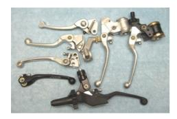
Here is an array showing the development in the ARC family. The top left is the first lever ever produced. It has Frankenstein springs on the outside to make it work. It was crude but proved that the concept was valid. Different lever shapes with folding and rotating concepts have been tried. We have scrapped more ideas than most companies ever bring to market.
