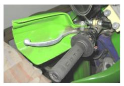
This is my '97 KLX300 dual sport bike. I just use it for transportation when I go camping so it does not get the "factory love" when it comes to levers. I like the clutch lever away from my fingers when fully disengaged. This is a perfect example of the need for the ARC folding lever. You can see how far forward I had to bend the lever to achieve the position that I liked. I usually broke one out of three when doing so.
