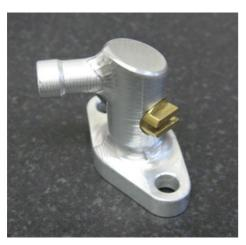
This is a close up of a gas valve. Not just any valve. I was at the Suzuki SX track one day when they were working on Rickys' bike. When removing the tank, the gas line was pinched with those doctor pinchers. I asked why and the answer was there was no room for a valve. He rode so hard that he boiled the fuel no matter how much insulation was used. They had to move the fuel supply to the rear of the tank by the carb and there was little room for a valve.
