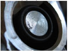
Notice the rings on the face of this brake master cylinder piston. This is the surface that the cam/thumb on the brake lever contacts and rubs on. When clean and greased it works smooth for a while. Dirt starts attaching to the lube and creates a gritty paste that wears out the parts. Our **brake levers** & clutch levers for the cam/thumb style master cylinders levers have a ball bearing at the contact point for smooth consistent operation.
