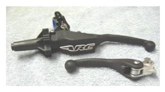
Our current gear is cutting edge technology for today. The new composite levers look factory and have a better feel than an aluminum blade. The shape of the lever where your fingers touch is the refinement from all the custom shapes we have done for top riders over the years. They are lighter by about 45% and can take a lot more abuse than conventional aluminum levers.
