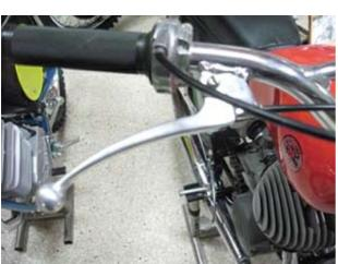
In the late '60's most of the brands went to aluminum for weight savings. This CZ was one of the first while still retaining the welded mount. There was no adjustability for placement on the bar. You rode what was there with no options. Also note that there is no cable adjustment at the lever. If you needed an adjustment you had to go to the pits and open the tool box.
