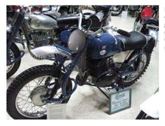
Here are a pair of Greeves, a 250 and 380. This was another brand of competitive 2-strokes. The fenders are worthy of a battle ship with the giant brackets and bolts to retain the aluminum fenders. These bikes also used steel levers with the innovation of using a clamp to attach the perch to the bars. That may seem small now but on those bikes the ability to move the levers where you wanted them was huge.
