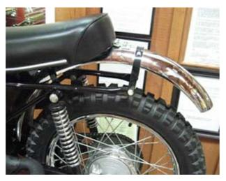
Not all of the old bikes were made by artists. Check out this DKW with a CHROME STEEL fender that has enough bracketry to withstand a force 5 tornado. I really like the door hinge that is right behind the seat making a double steel bracket support within 3". When something is heavy you need heavy stuff to retain it. The DKW 125 weighed in at close to 230lbs dry and had something like 17 horsepower.
