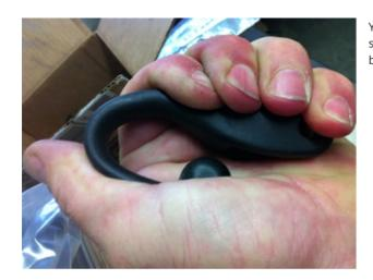
You can bend an aluminum lever like this too. When an aluminum lever is straightened it will get you through the weekend but will have wrinkles and be much weaker from the abuse.
