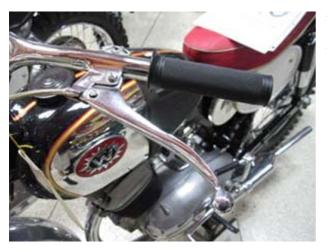
The hand craftmanship and love that went into the making of the early bikes is true art. I personally do not wish to race a tractor on a motocross track though. This White 2-stroke was way lighter than the 4-strokes of the day but 250lbs is still a heavy ride. Note the welded steel perches and steel levers that were the standard. A quick adjust was not thought of since nothing about these bikes was quick.
