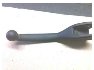
Here is a copy of our latest composite clutch lever. Look at the blade portion where your fingers contact the lever. It is smooth and shiny with no suface defects.
