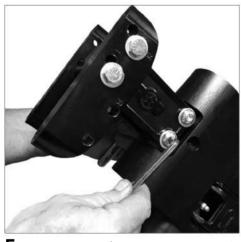
Torque with 3/8" allen wrench and socket to 25ft.-lbs.
