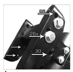
Adjust the fairing mount wing bolts based on your wheel size (26", 26x", 30"). 26X is the most common fitment for 26" wheels
