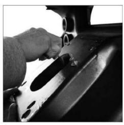
Attach inner fairing to the front of the mount and tighten bolts.
