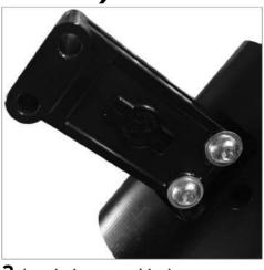
Attach the center block mounts to the neck with 3/8-16z3-1/2 bolts, washers, and lock nuts.
