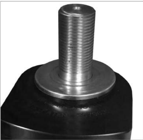
34 Re-use the stock top dust cover and place it on top of the bearing and washer.
