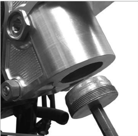
22 Make sure to grease your bearing races before installing set screws. Insert lower set screw into bottom of the Bolt on Neck.
