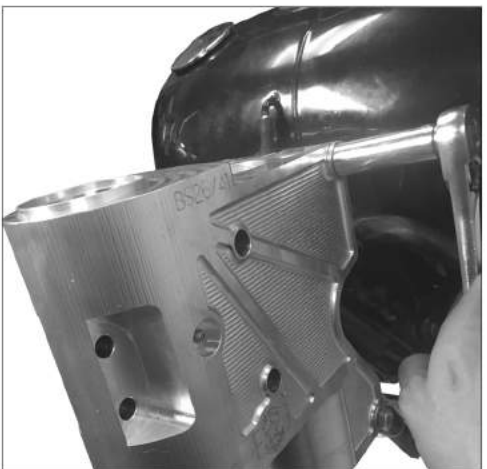
27 Torque the upper and lower mounting bolts to 30ft/lbs.
