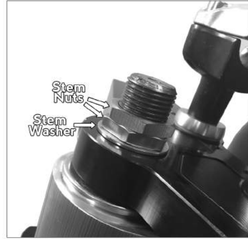
36 Install first stem nut. Tighten the nut slowly and wiggle the trees until the bearing clicks. Tighten until the clicking stops plus an extra 1/4 turn. Tighten the second stem nut against the first.
