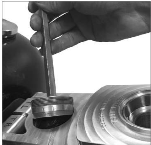
23 Insert upper set screw on the Bolt on Neck. Torque upper and lower set screws to 80ft/lbs.
