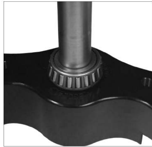
30 Pack bearings through with grease and slide through the stem of the lower tree.
