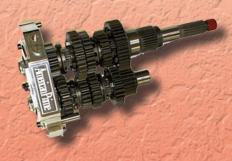
1216-0001 COMPLETE COMP MASTER™ 6 SPEED CLOSE RATIO LSD GEAR SET WITH TRAP DOOR ASSEMBLED ON MAINSHAFT & COUNTERSHAFT. INCLUDES SHIFTER DRUM, SHIFTING AS-SEMBLY, SHIFTER FORKS, BEARINGS & CHROME TOP COVER. FITS LSD 5 SPEED BIG TWIN TRANSMISSIONS EXCEPT 2006 DYNA MODELS & AFTERMARKET 6 SPEED TRANS. CLOSE RATIO 2.94:1 FIRST GEAR; SECOND GEAR 2.21; 0.860:1 OVERDRIVE SIXTH GEAR. FORGED AND BACK CUT GEARS FOR POSITIVE SHIFTING.
