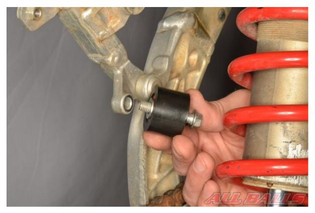
Install the new chain rollers with the washer against the frame.
