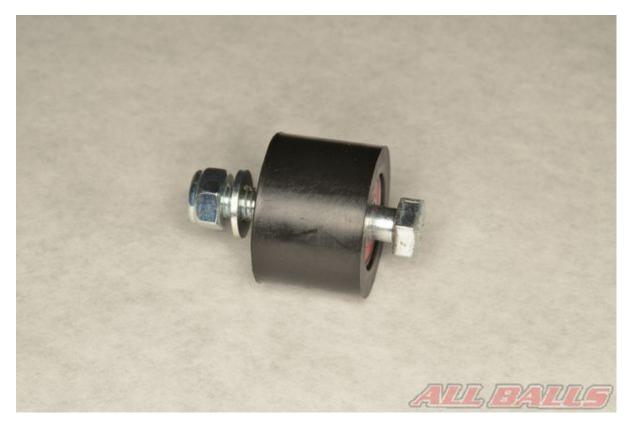
Layout the components in an organized manner for easy installation. Note: wait to do this until the old parts are removed and you are ready to begin installing the new components.
