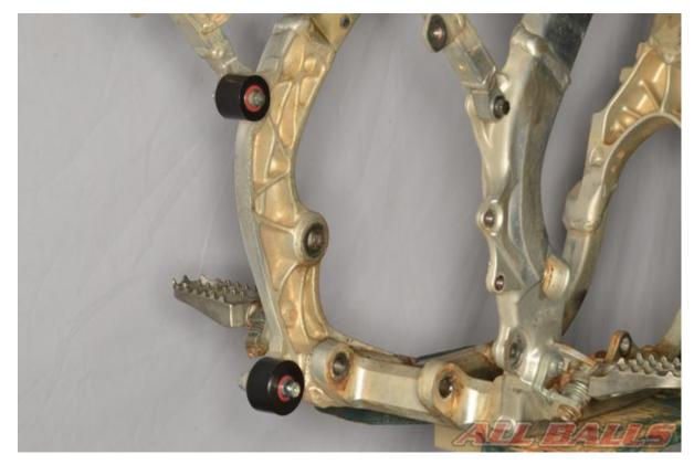
Tighten the fasteners securely. Follow the torque specifications in the vehicle's service manual. Make sure the rollers spin freely.
