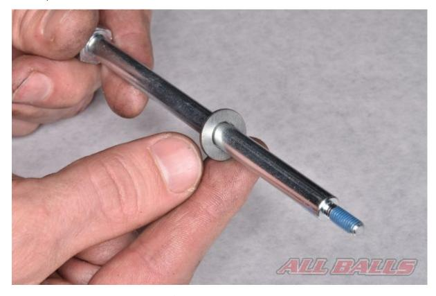
Install the plain washer onto the jack shaft bolt.
