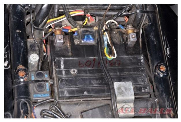
Connect the negative battery lead.
