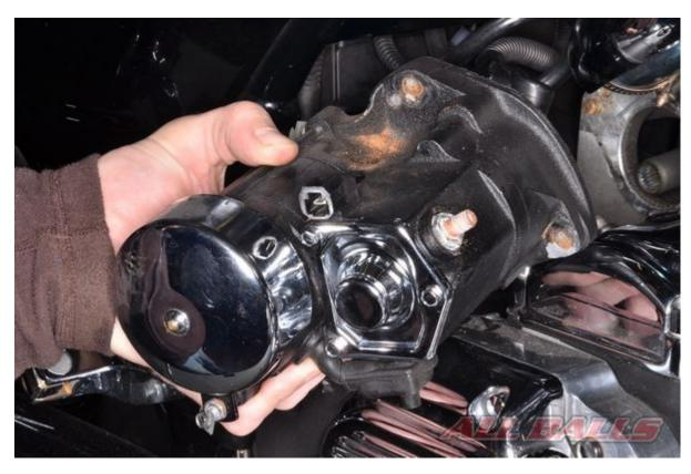
Remove the starter motor.
