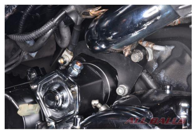
Remove the 2 starter motor mounting bolts. Some models may require the removal of an exhaust bracket.
