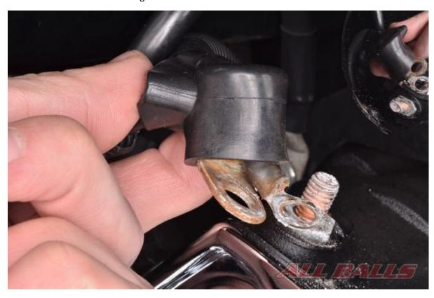
Pull back the rubber boot, remove the lock nut and free the starter motor cables.
