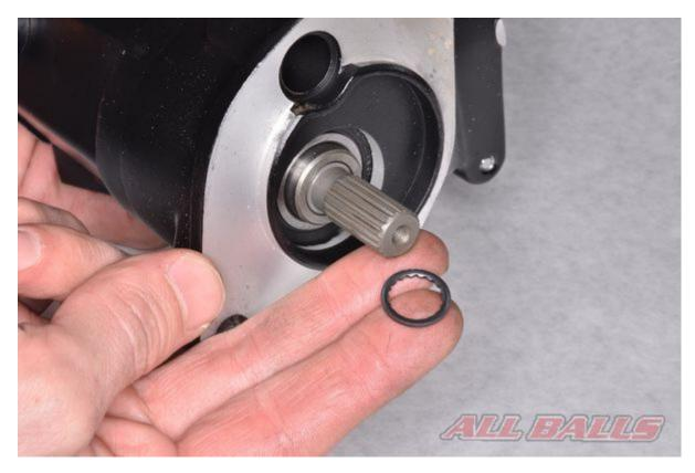
Install the the splined washer onto the new starter motor, a small dab of grease will help hold it in place. Apply a thin coat of grease to the starter motor splines.
