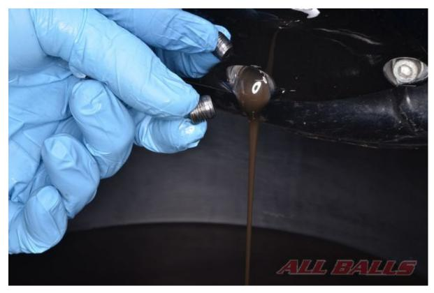
Remove the drain plug and allow the primary oil to drain completely.
