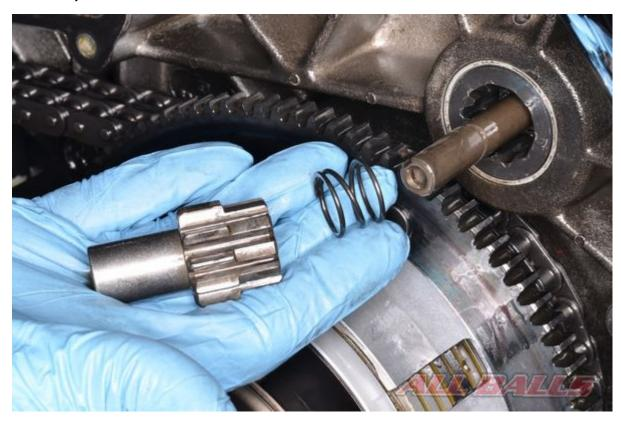
Remove the pinion gear and spring, and check for any damaged teeth on the starter driven gear on the clutch basket. Replace the components as necessary.
