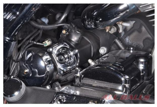
Locate the starter motor on the right side of the machine.
