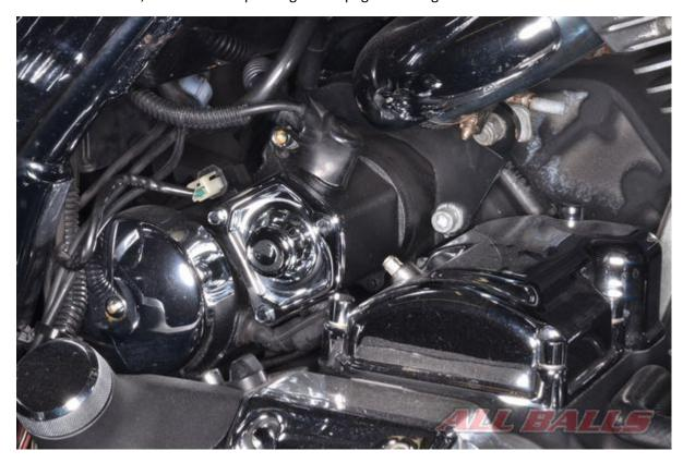
Connect the solenoid lead and battery cables, pull the rubber boot over the cables.
