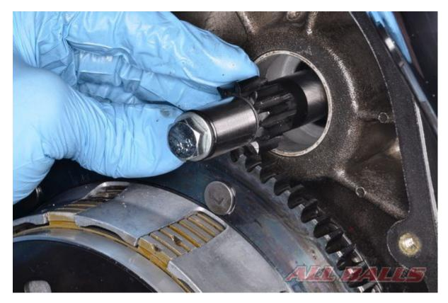
Install the bolt into the jack shaft, hold the jack shaft with a suitable tool and tighten the bolt to 5 ft. lbs.
