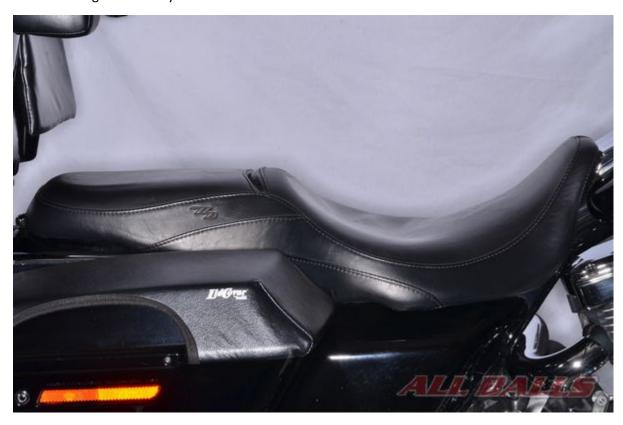
Install the seat and tighten the bolt securely to the manufacturers specification.
