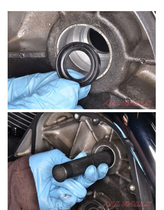
Install the new jack shaft oil seal into the left case half until it is fully seated.
