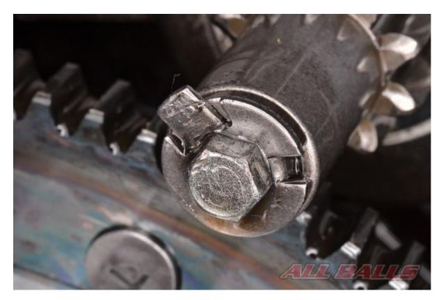
Bend the tab on the lock washer.
