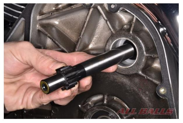
Install the new jack shaft onto the starter motor shaft, carefully guide it through the oil seal. Make sure it fits correctly- you will feel it press against the spring.
