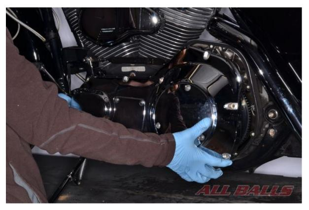
Remove the mounting bolts and the primary chain case cover.
