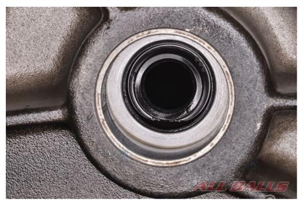
Drive out the old jack shaft oil seal and note the direction of the seal for installation.
