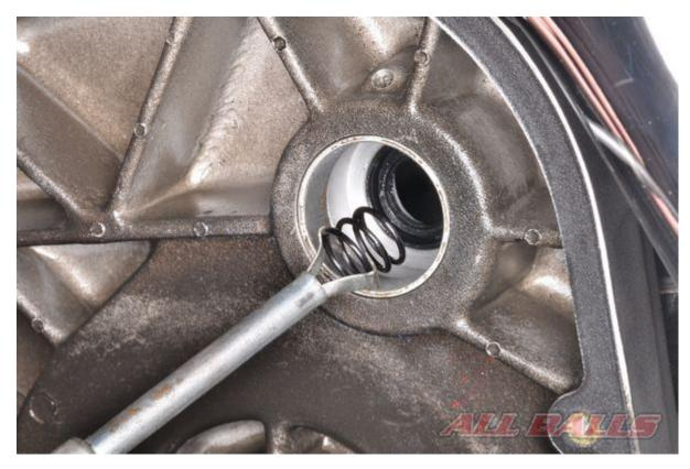
Using a suitable holding tool, carefully place the spring onto the starter motor shaft. Avoid damaging the oil seal or dropping the spring.
