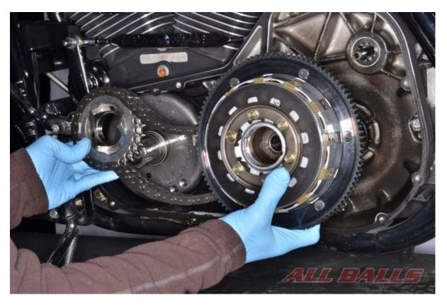
Follow the manufacturers instructions and remove the clutch and primary chain as an assembly.
