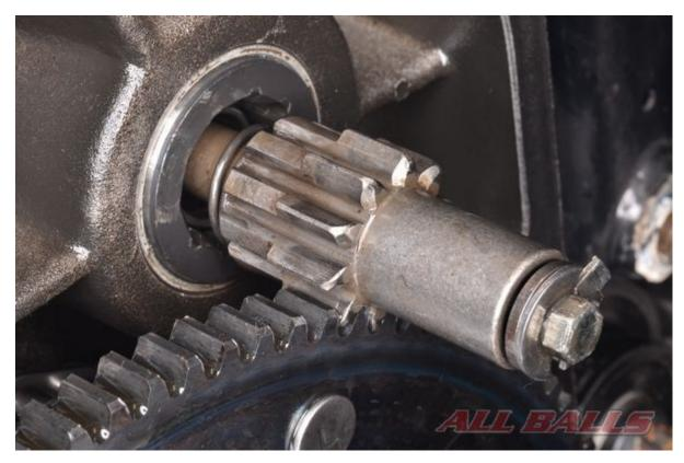
Extend the pinion gear so it can be held by the clutch driven gear and loosen the jack shaft bolt. Wrap the pinion gear with a rag and hold it with pliers if needed to keep it from turning when the bolt is loosened.
