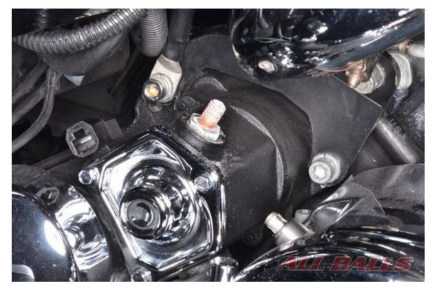
Install the new starter motor onto the engine. Tighten the bolts to specification with a toque wrench.
