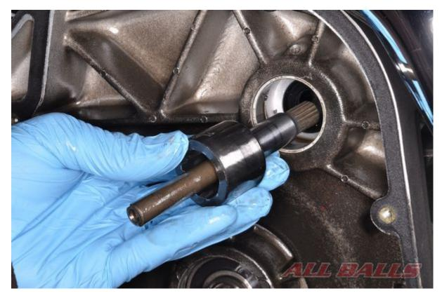
Remove the coupling and the old jack shaft.
