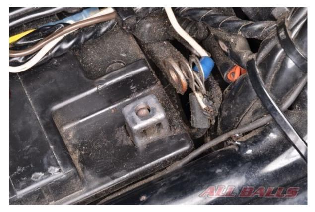
Disconnect the ground lead from the battery.
