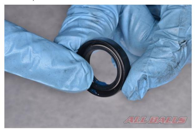
Apply a thin coat of grease to the new oil seal lips.
