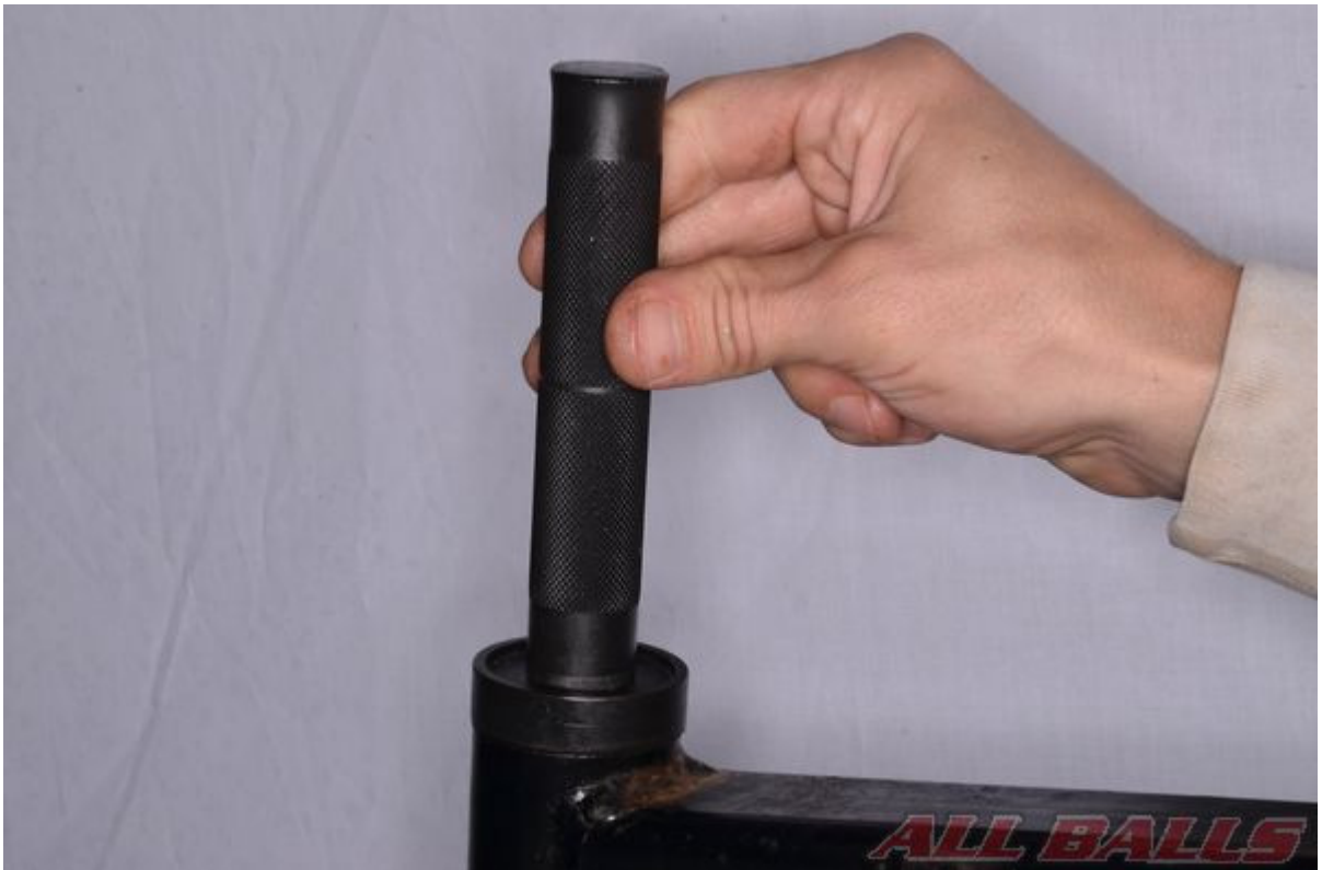
Install the dust seals into the swingarm.
