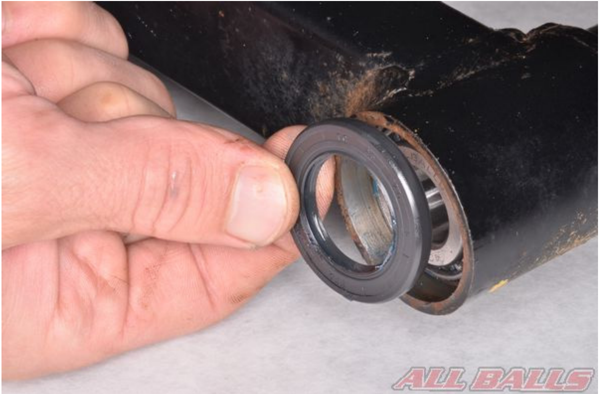
Install the dust seals into the swingarm.
