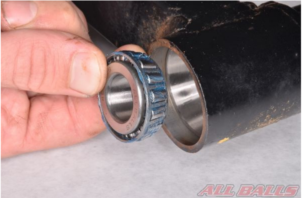
Install the swingarm bearings into the races.
