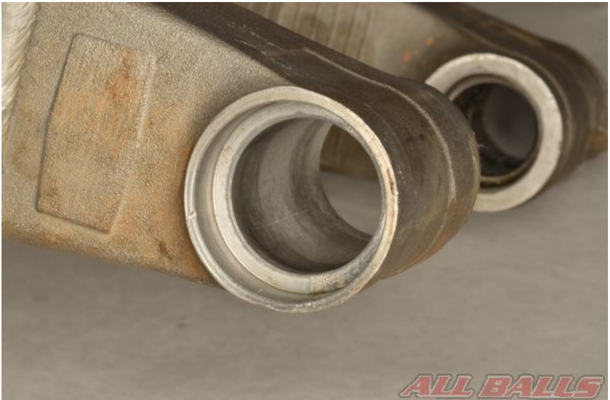
Inspect the bearing bores for wear and damage. Make sure the bores are free of damage or burrs that may cause the new bearings to hang during installation.
