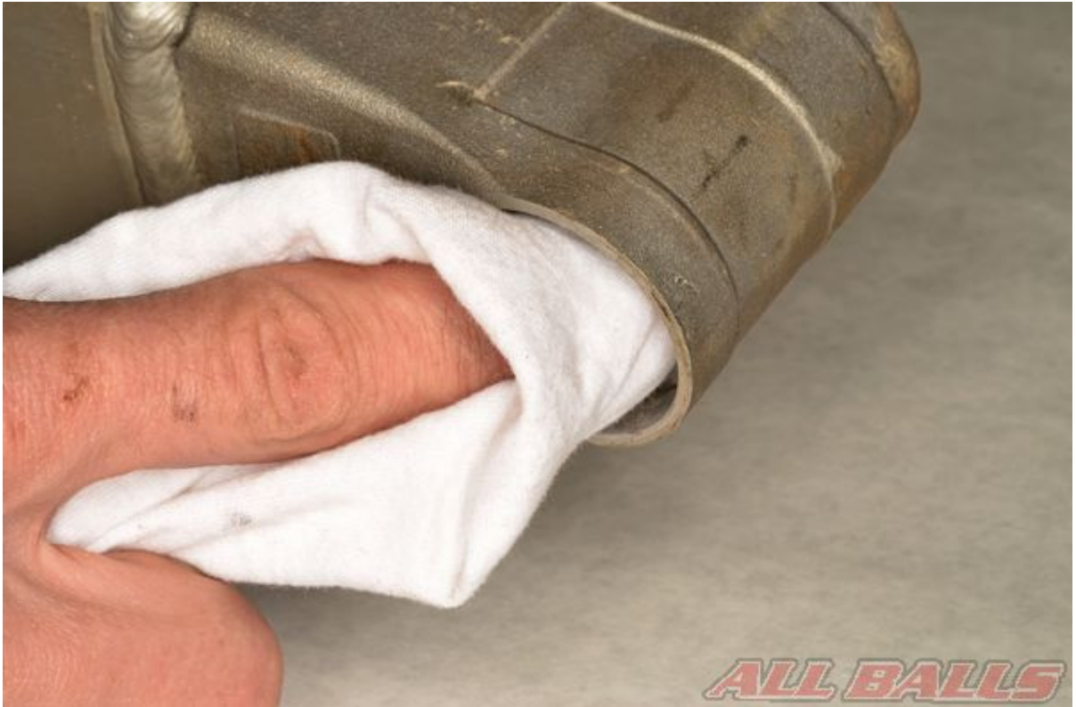
Clean away all of the old grease, grime, and rust from the bearing bores.
