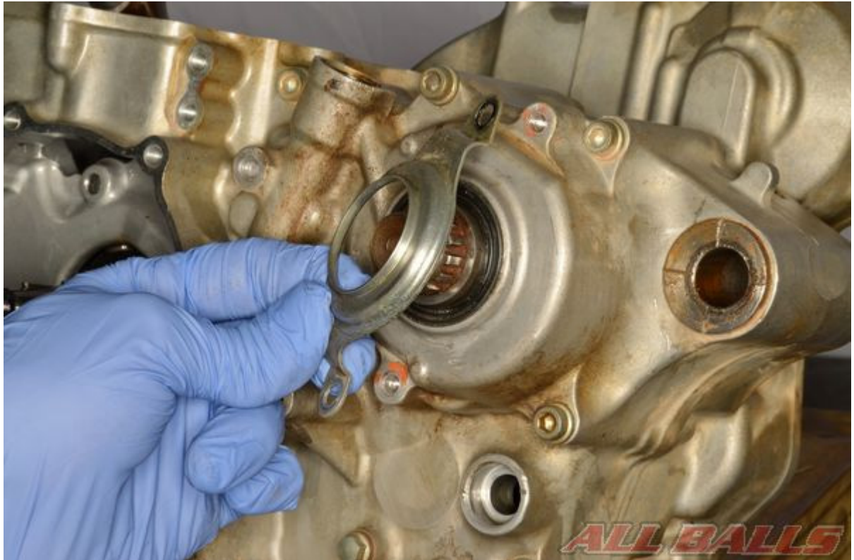
Some models have a countershaft seal retainer. Remove the countershaft seal retainer.
