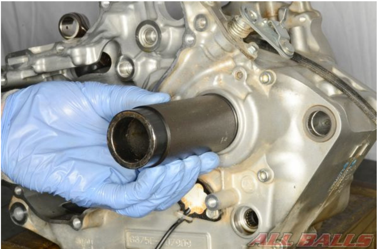
Press in the the seal by hand in with an appropriate driver or a socket with the same outside diameter of the seal.
