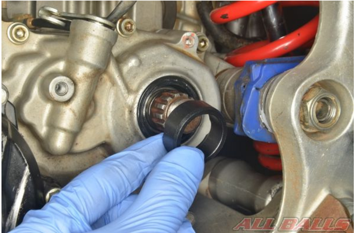
Install the new countershaft bushing.
