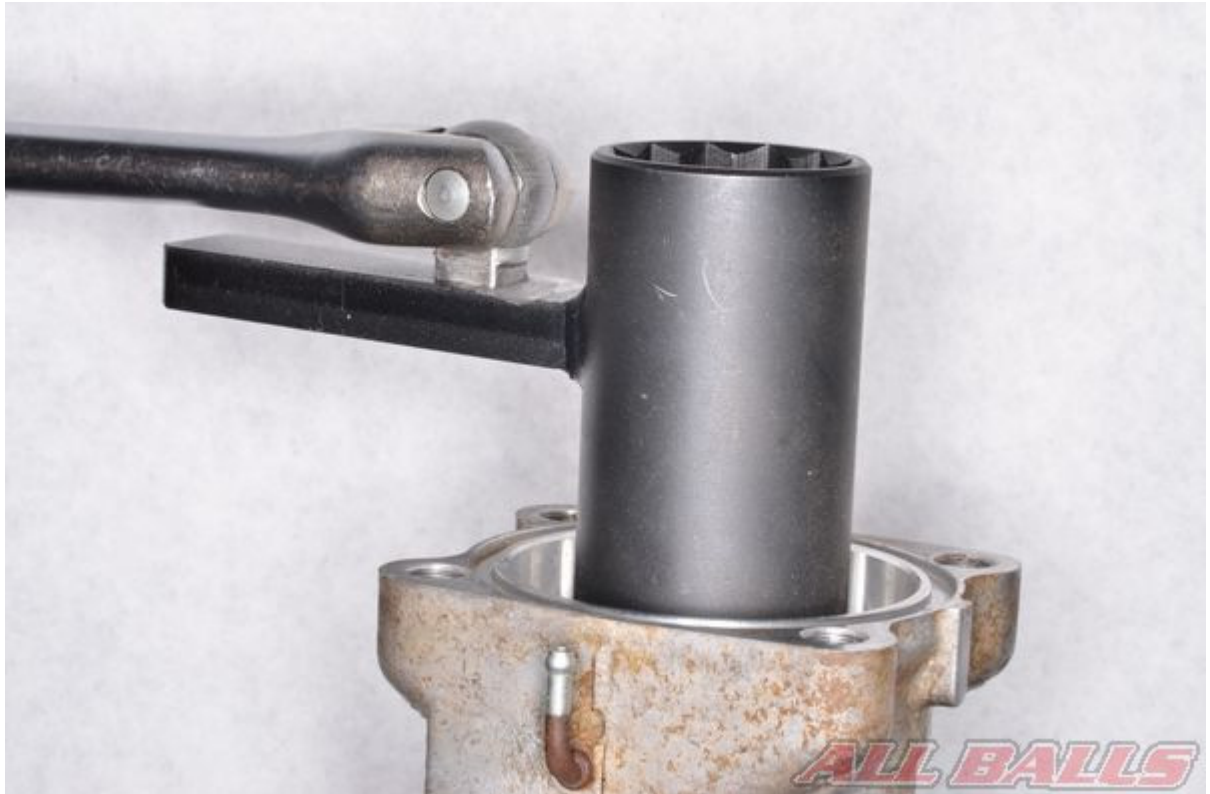
Loosen the inner lock nut with the special lock nut wrench.
