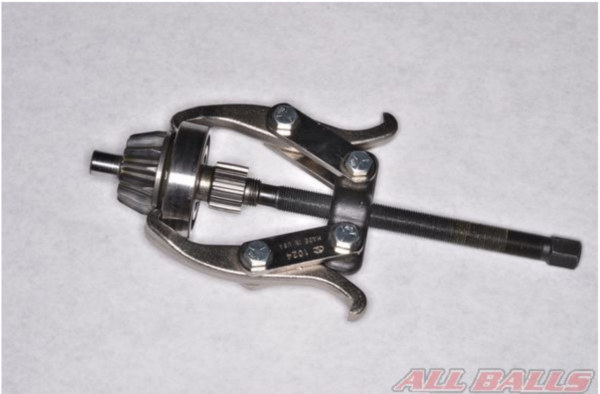
Use a bearing puller tool to remove the bearing from the pinion gear shaft.
