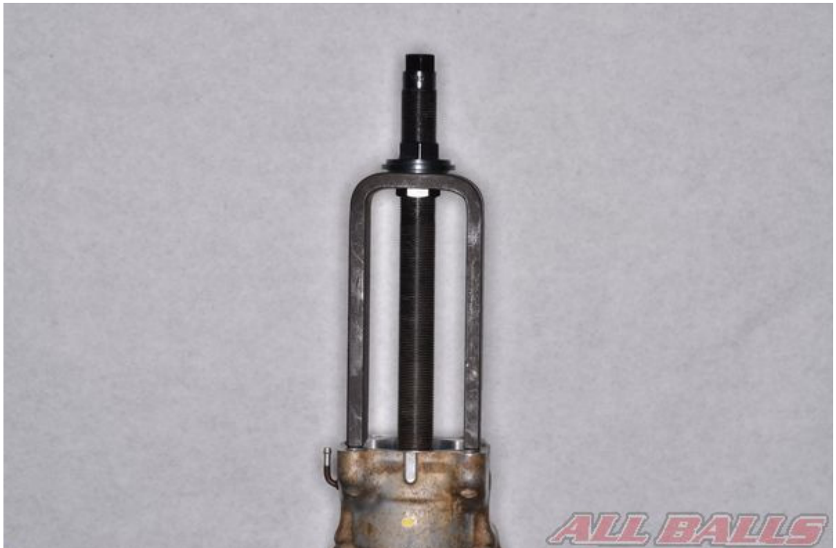
Use a special puller tool to remove the pinion gear.
