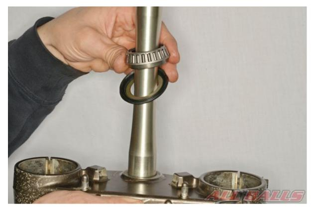
Fit the new dust seal and lower bearing onto the steering stem.
