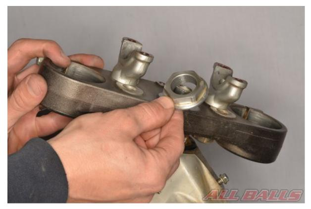
Remove the steering stem nut.
