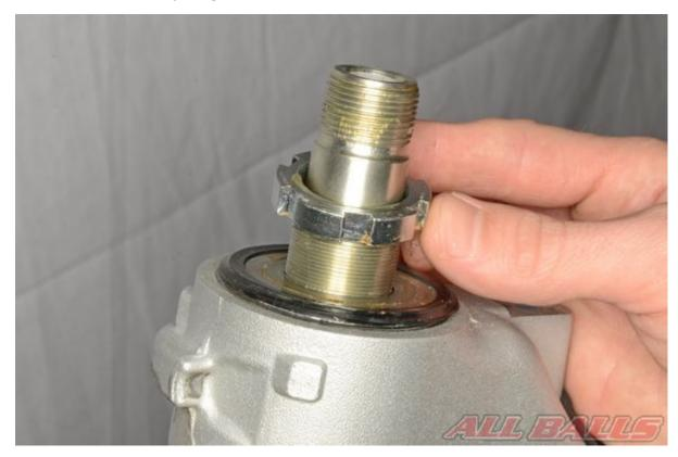
Make sure to support the lower triple clamp with your free hand, as it can fall out with the nut removed.
