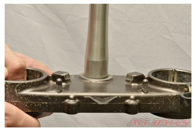
Make sure the steering stem is clean and in good condition to accept the new bearing and dust seal. Remove any burrs from the stem that might prevent smooth bearing installation.
