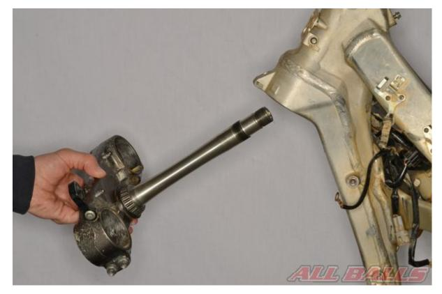
Remove the lower fprl clamp and steering stem from the steering head.
