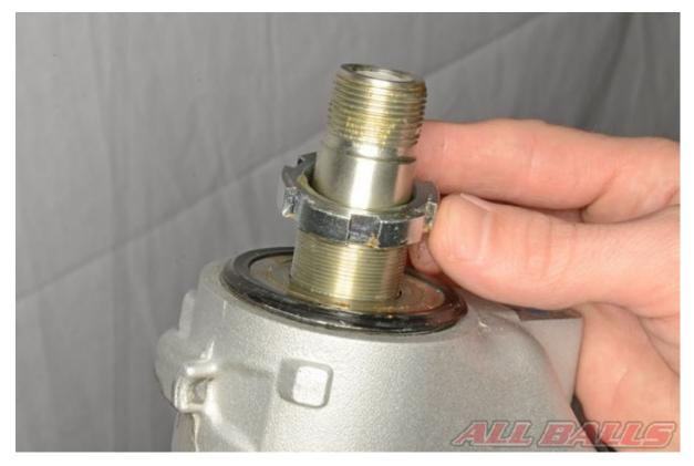
Thread on the adjusting nut.
