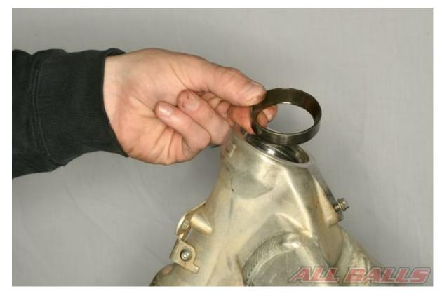
Remove the upper and lower bearing races.
