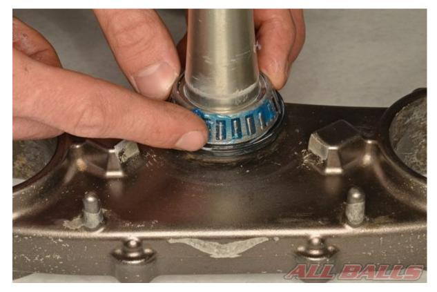
Lubricate the bearings with grease.
