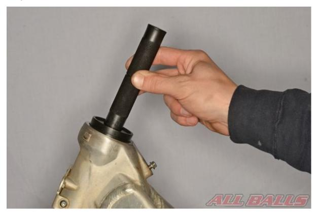
A suitable bearing race driver may also be used to install the races into the steering head. Make sure the driver fits the race correctly and take care to drive race in straight.
