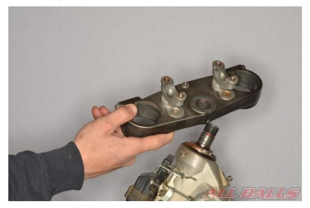
Lift the upper fork clamp off the steering stem.
