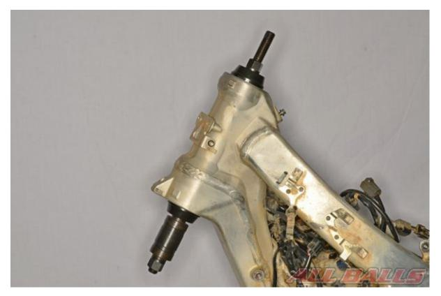
Use an appropriate bearing race installation tool to install the races into the steering head of the frame. Makes sure the bearing races go in straight. Do not apply pressure to the tapered portion of the races to prevent damage.
