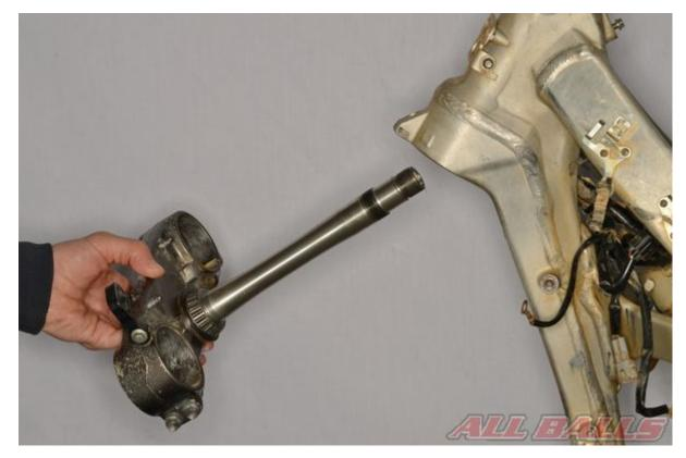
Fit the steering stem into the steering head of the frame.
