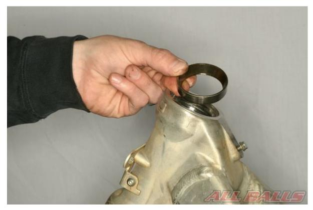
Install the new bearing races into the steering head of the frame.
