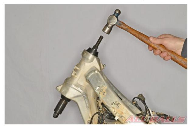
After the bearings are pulled in hit both ends of the threaded rod with a hammer to fully seat the bearings.
