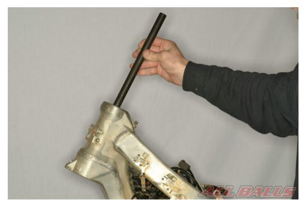
Remove the steering bearing races with a steering bearing race remover tool.
