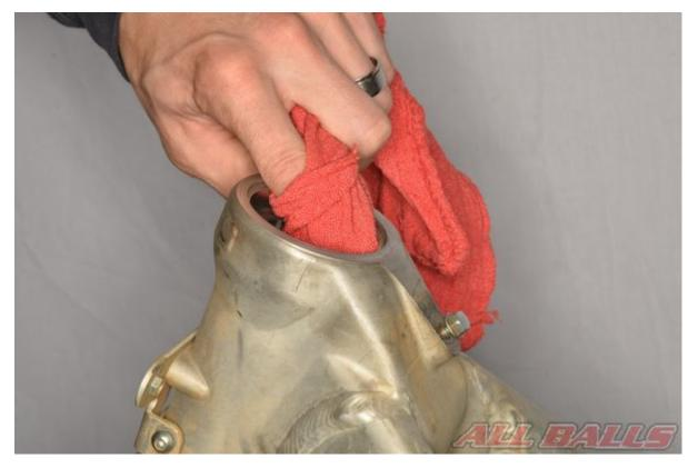
Clean away all of the old grease, grime, and rust from the bearing bores. Inspect the condition of the steering head in the frame. Remove any burrs that may inhibit the installation of the new bearing races.
