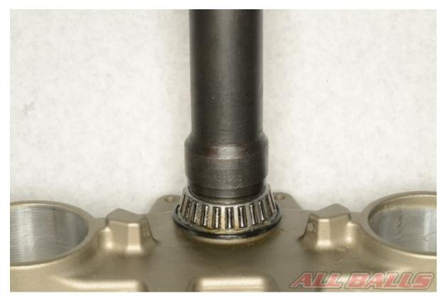
Make sure the bearing installer tool or pipe, only makes contact with the inner race of the bearing. Pressing on the cage of the bearing will distort it and may cause binding in your steering.
