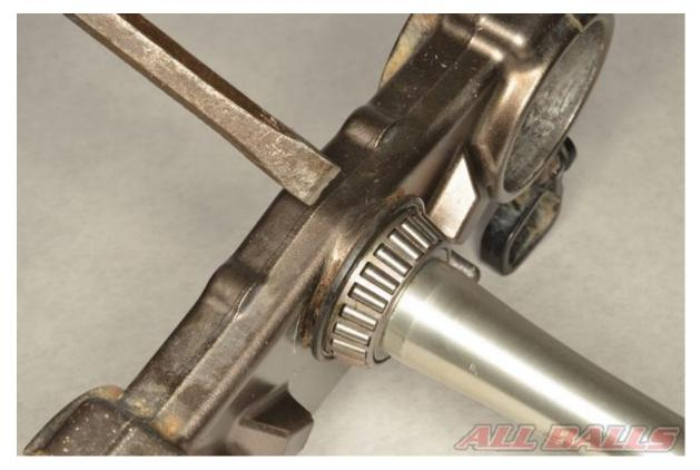
Remove the lower stem bearing by tapping a chisel between the bearing and the triple clamp. Work your way around until the bearing pops free.
