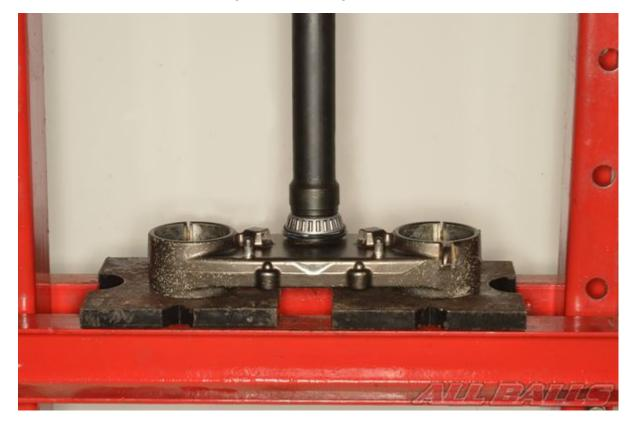
Use a press with a steering stem bearing installer tool to install the lower bearing onto the steering stem.
