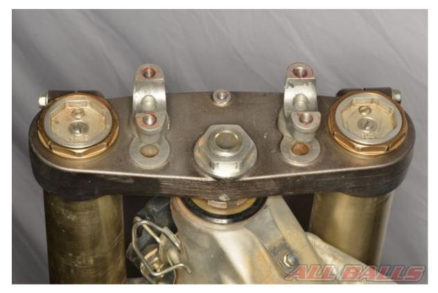
Install the forks and tighten the steering stem nut to specification.
