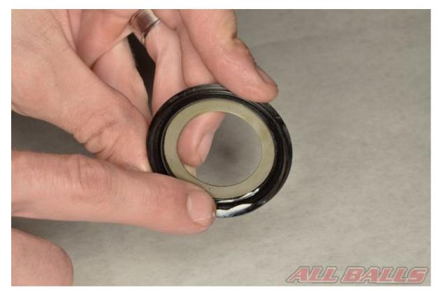
Lubricate the dust seal lips with grease.
