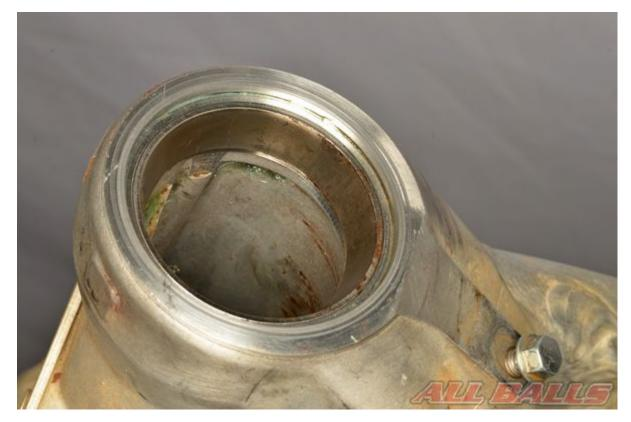
The bearing races are in the steering head of the frame. There are two races – one for the upper bearing and one for the lower.
