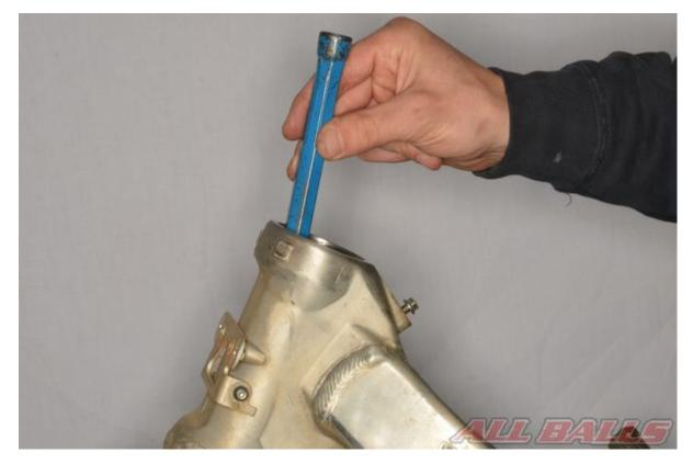
If a steering bearing remover tool is not available, remove the bearing races by knocking them out with a drift and hammer.
