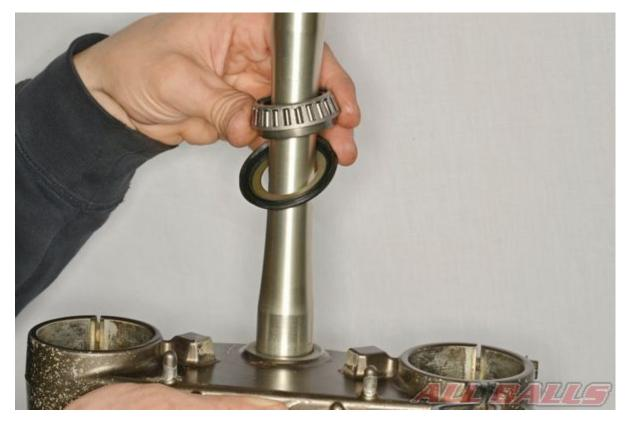
Remove the lower bearing and dust seal.
