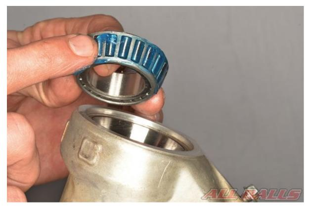
Install the upper bearing into its race.
