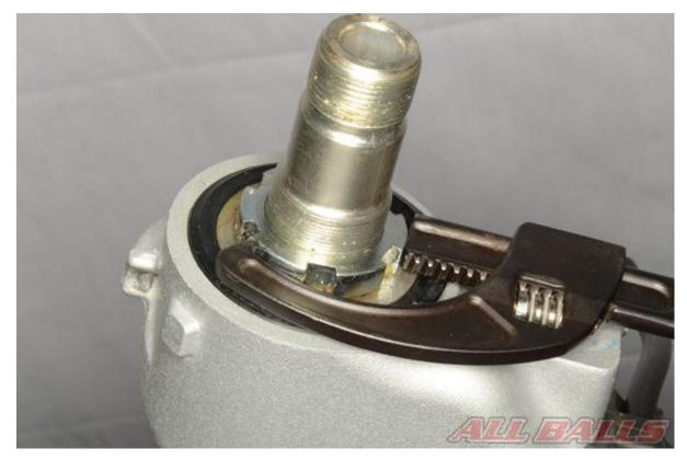
Loosen and remove the adjusting nut.
