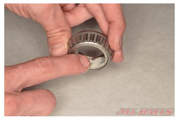
Apply a light coat of grease to the inside diameter of the lower bearing to aid installation.
