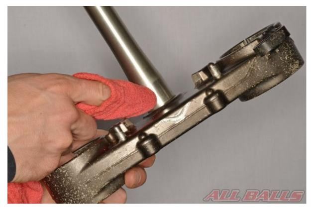
Clean away all of the old grease, grime, and rust from the bottom of the steering stem.
