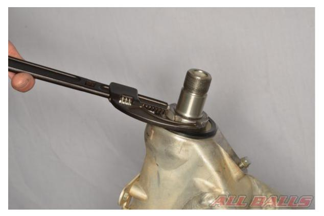
Tighten the adjusting nut with a pin spanner. Follow any specific adjusting nut instructions in the service manual
