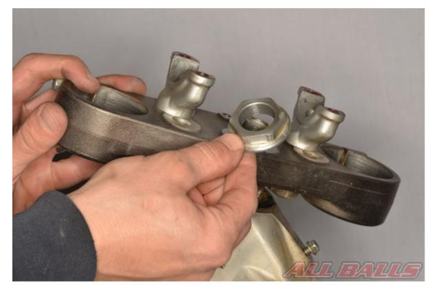
Install the steering head nut.
