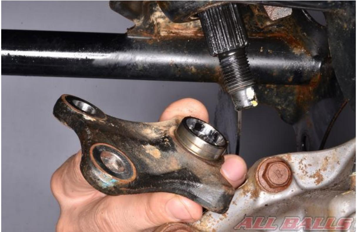
Align the splines correctly and install the pitman arm onto the steering stem.
