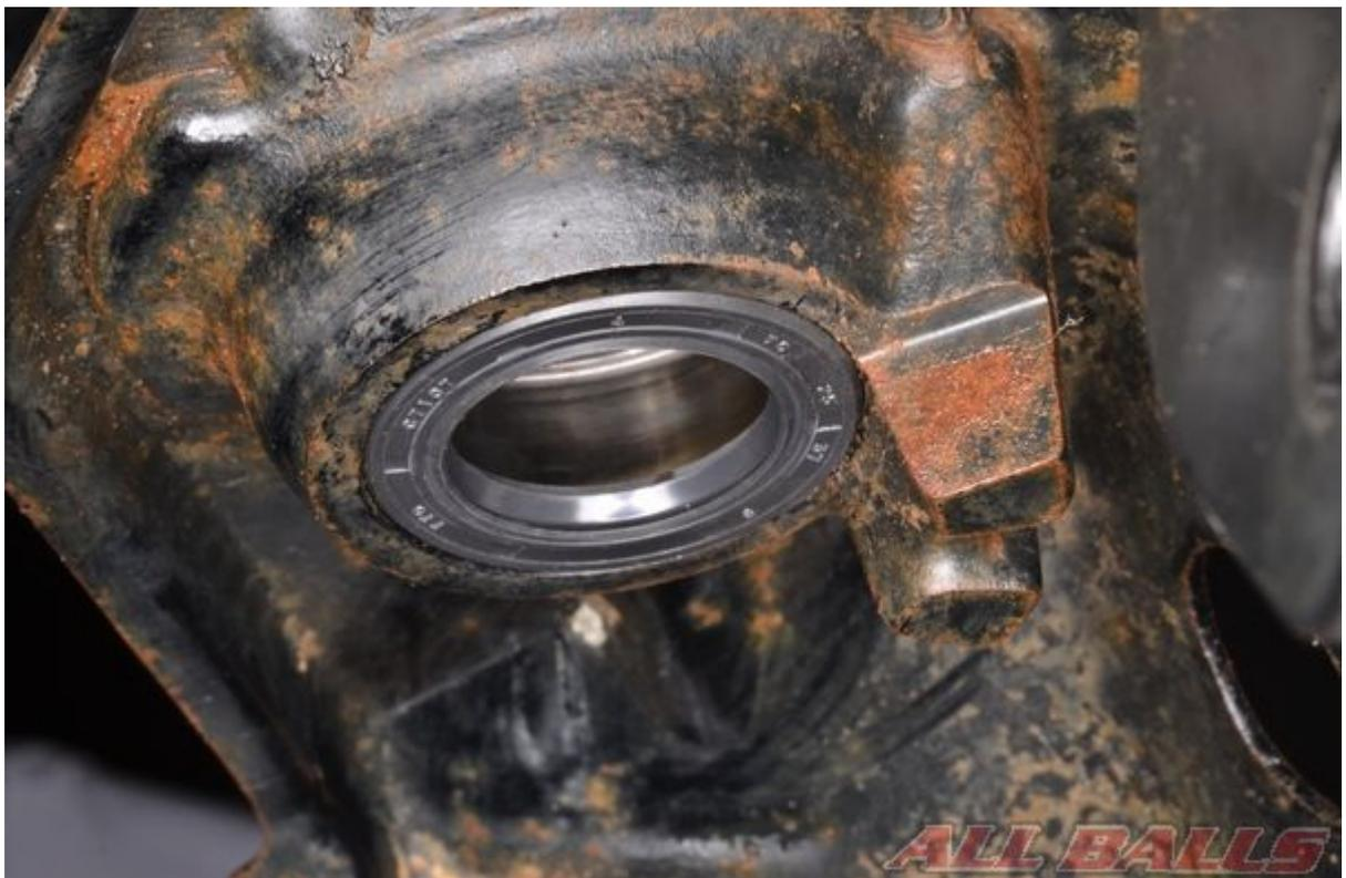
Press in the seals by hand or use a suitable driver that matches up with the outside diameter as the dust seal if needed.
