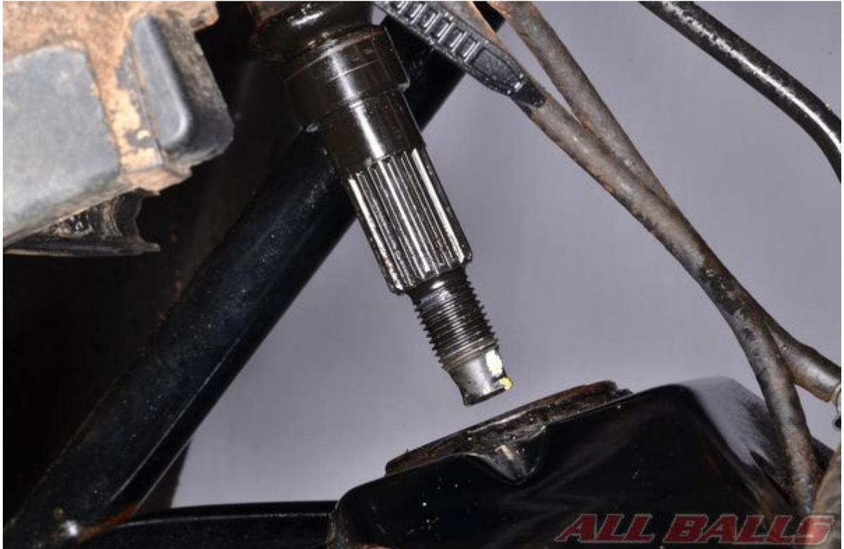
Lift the steering stem up and free it from the bearing and frame.
