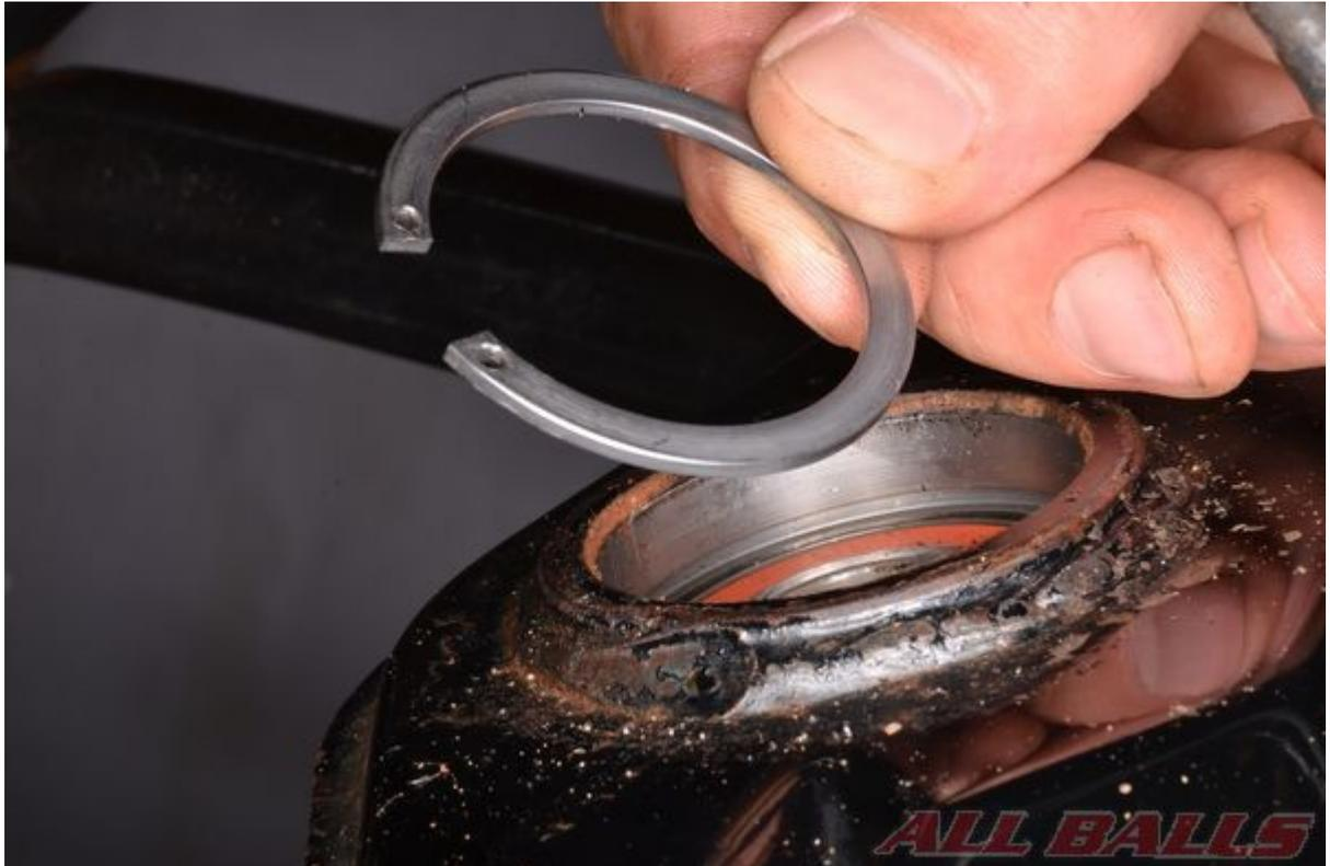
Remove the snap ring with snap ring pliers.
