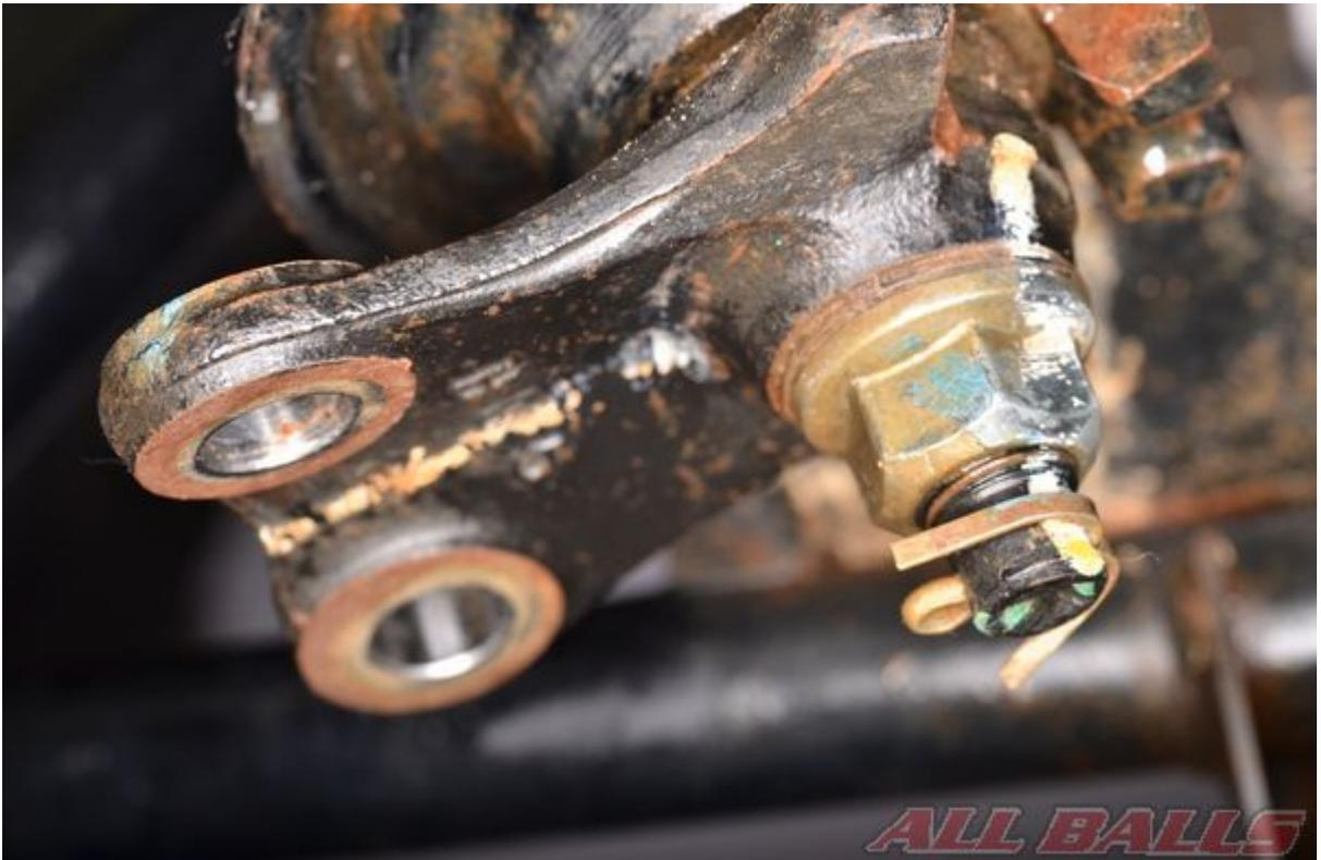
Install the the new steering stem nut cotter pin.
