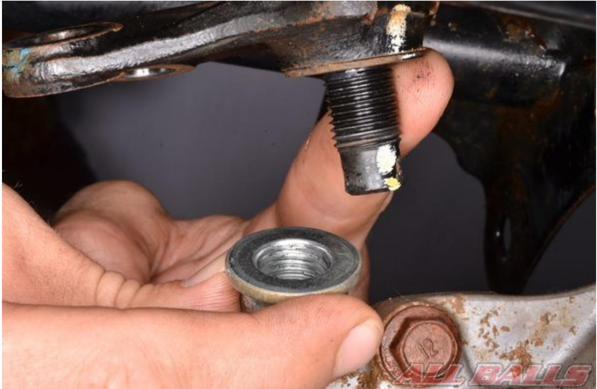
Install the washer and nut. Tighten the steering stem nut to specification.
