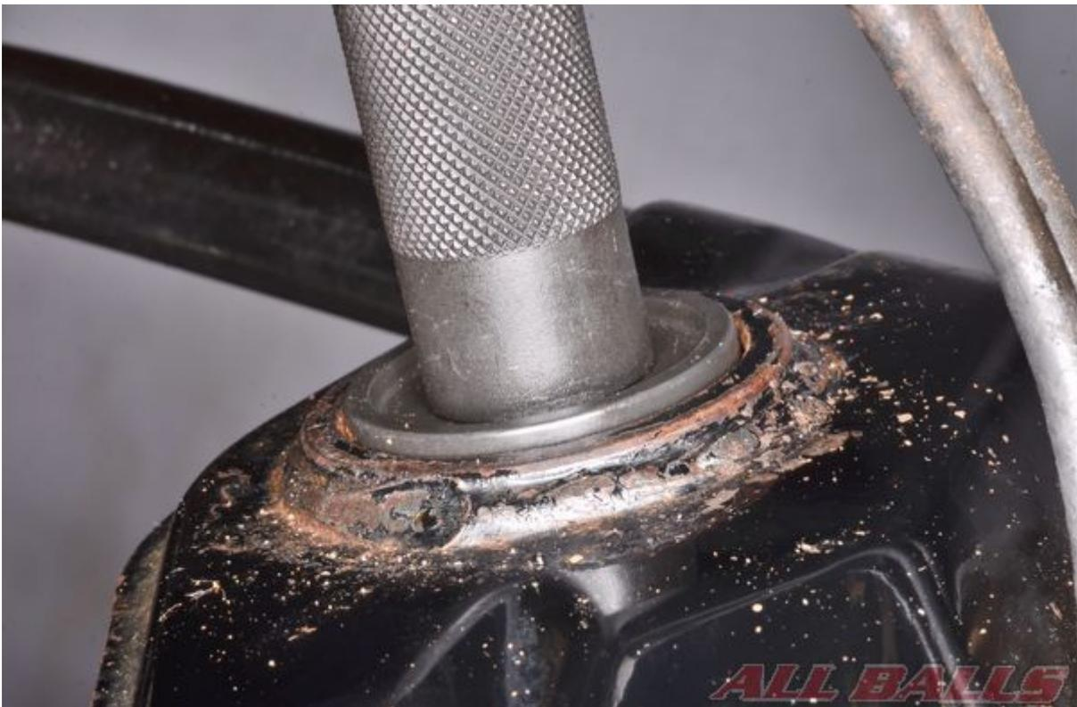
Drive the bearing into place with a bearing installer tool or a socket that matches up with the outer race of the bearing. Only press on the outer race of the bearing.
