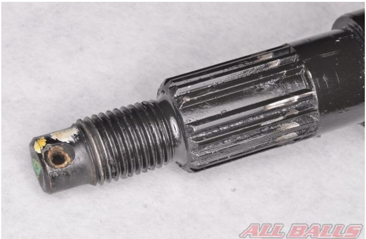
Clean the steering stem and inspect it for wear and damage. Replace the stem if it is bent or otherwise damaged.
