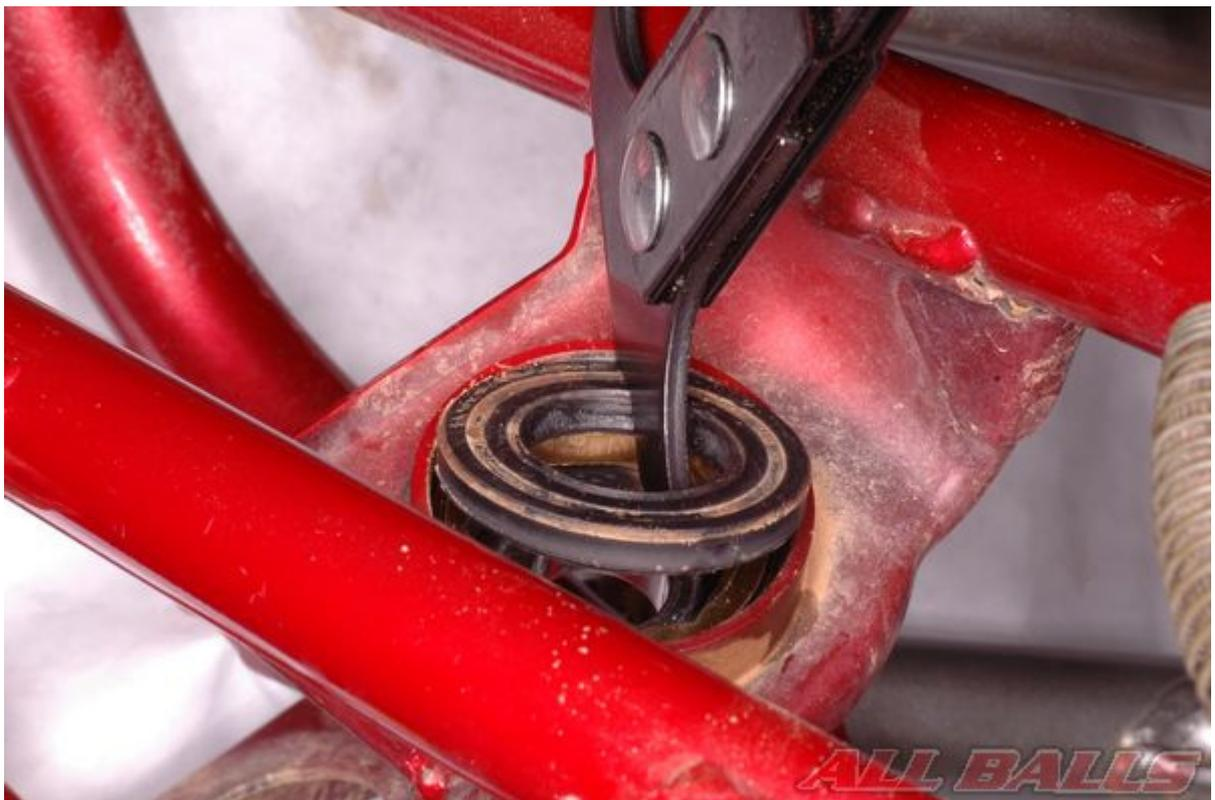
Remove the steering stem collars and dust seals.
