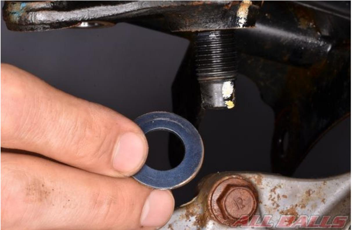
Remove the steering stem nut and washer.
