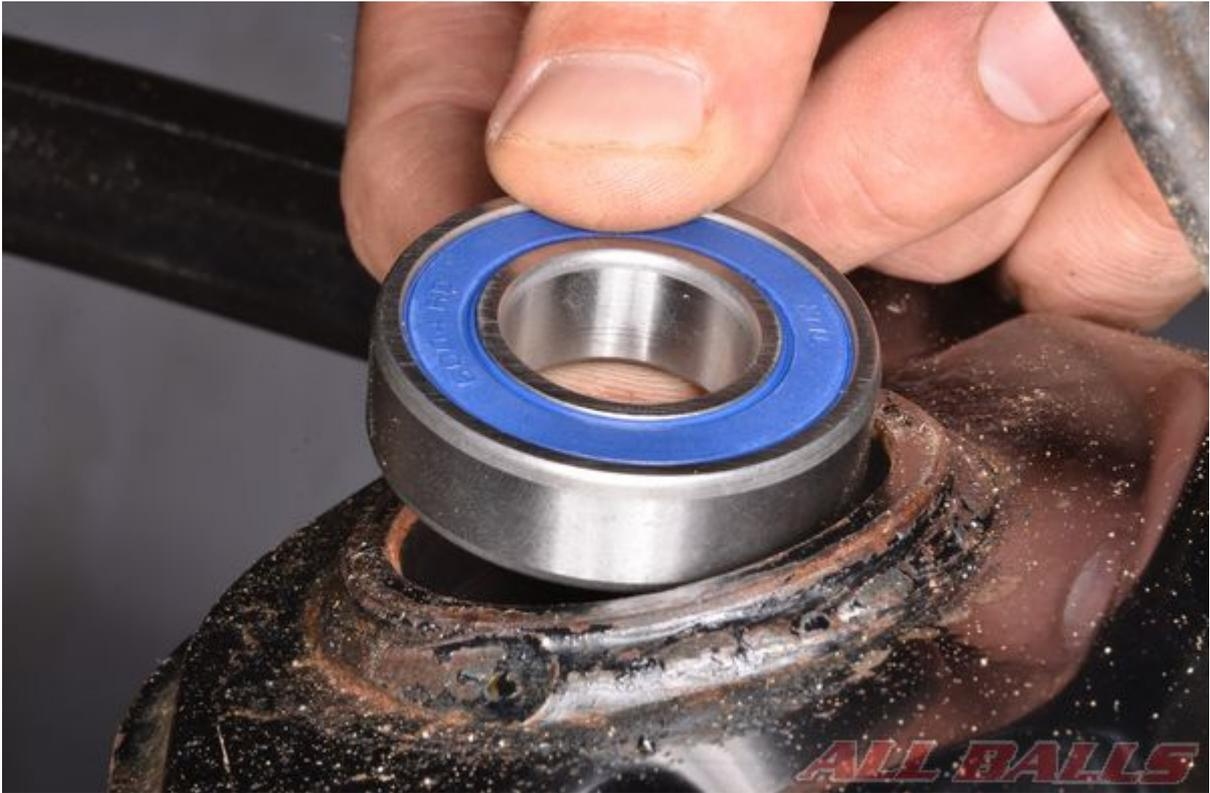
Heat the bearing area with a heat gun, take the bearing out of the freezer and install it into the frame.
