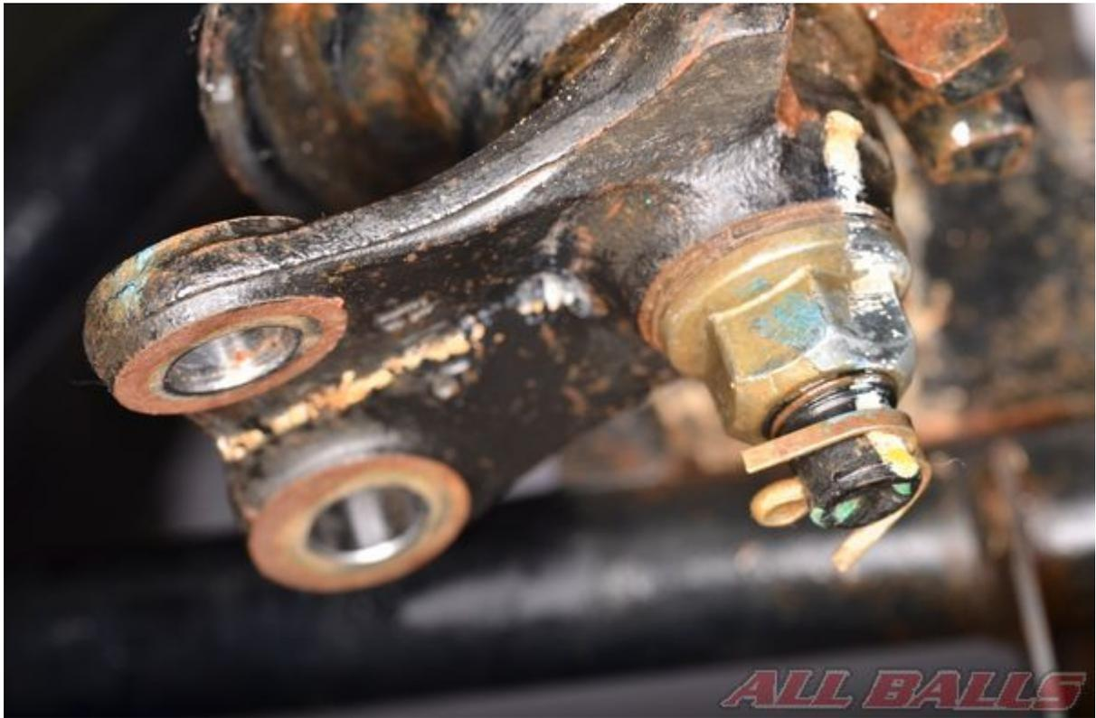
Disconnect the tie-rods from the pitman arm.
