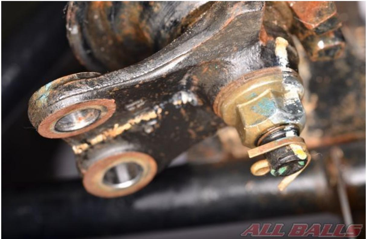
Disconnect the tie-rods from the pitman arm.
