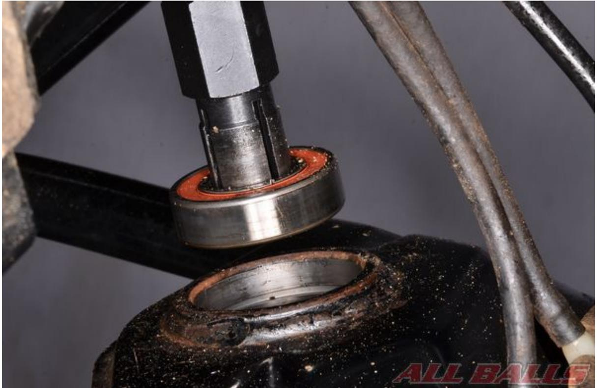
Use a suitable bearing puller to remove the steering stem bearing from the frame.
