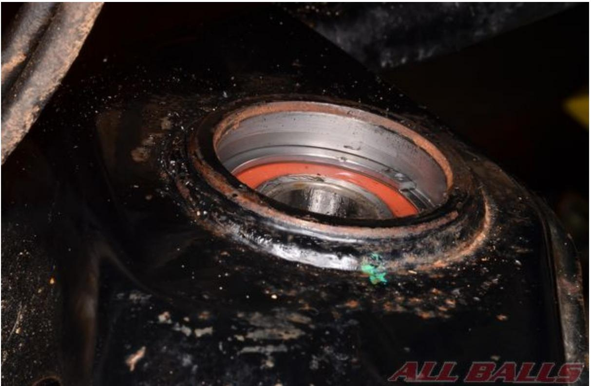
Install the snap ring into the snap ring groove with snap ring pliers.
