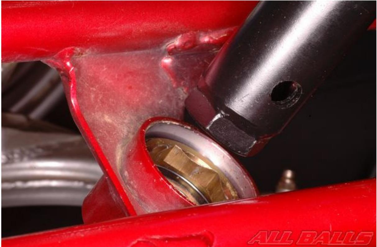
Install the steering stem bearing inner locknut if the bearing is secured in the frame in this manner. Tighten the inner locknut to specification with the special tool.
