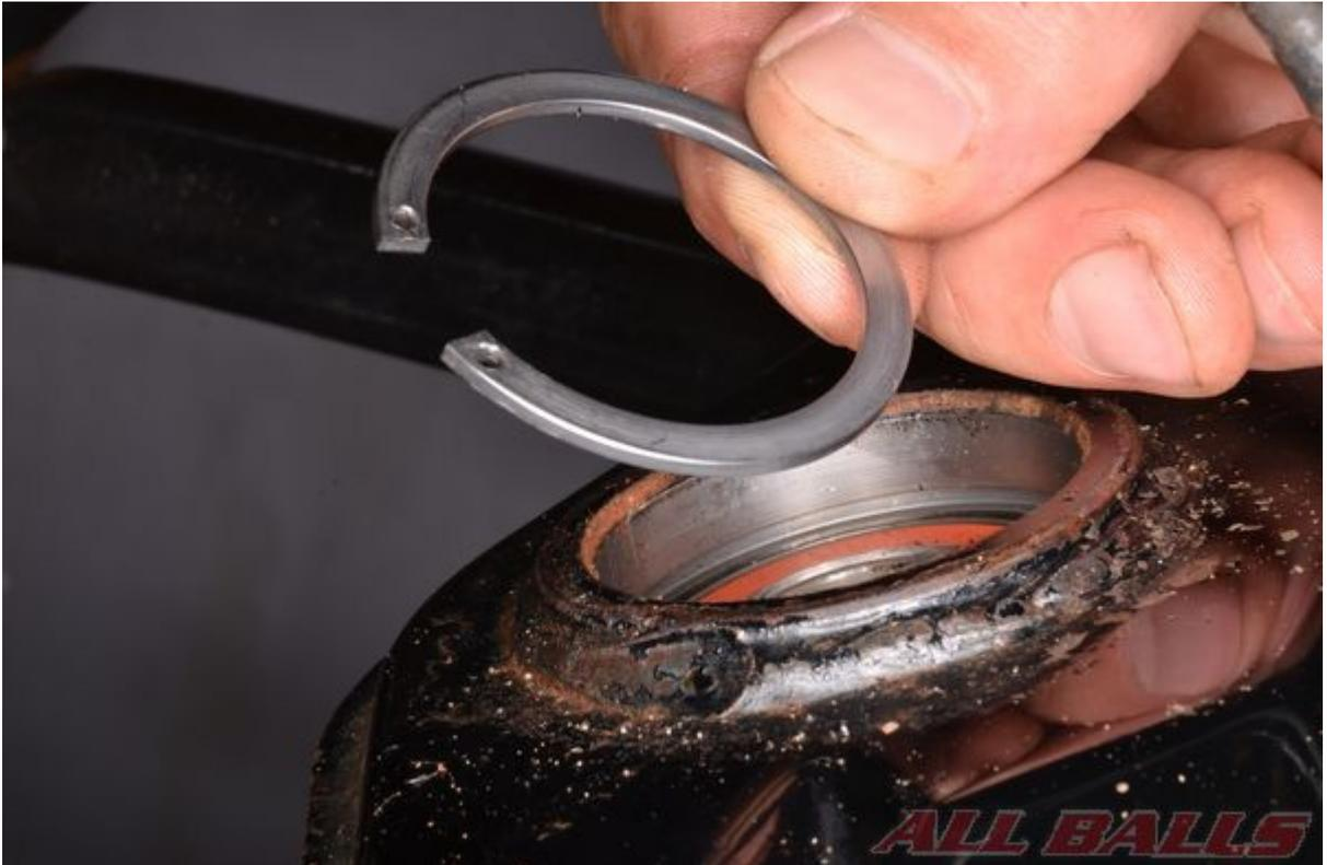
Make sure the bearing is fully seated. The snap ring groove should be visible if the frame requires a snap ring to secure the bearing.
