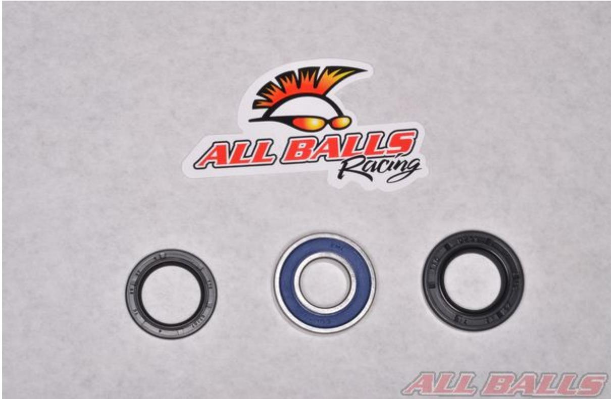
Remove the contents of your ALL BALLS RACING carrier kit. Layout the components in an organized manner for easy installation. Place the new bearings in the freezer for about an hour before installing them.
