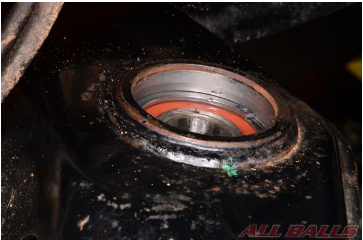
Some steering stem bearings are held in by snap rings.
