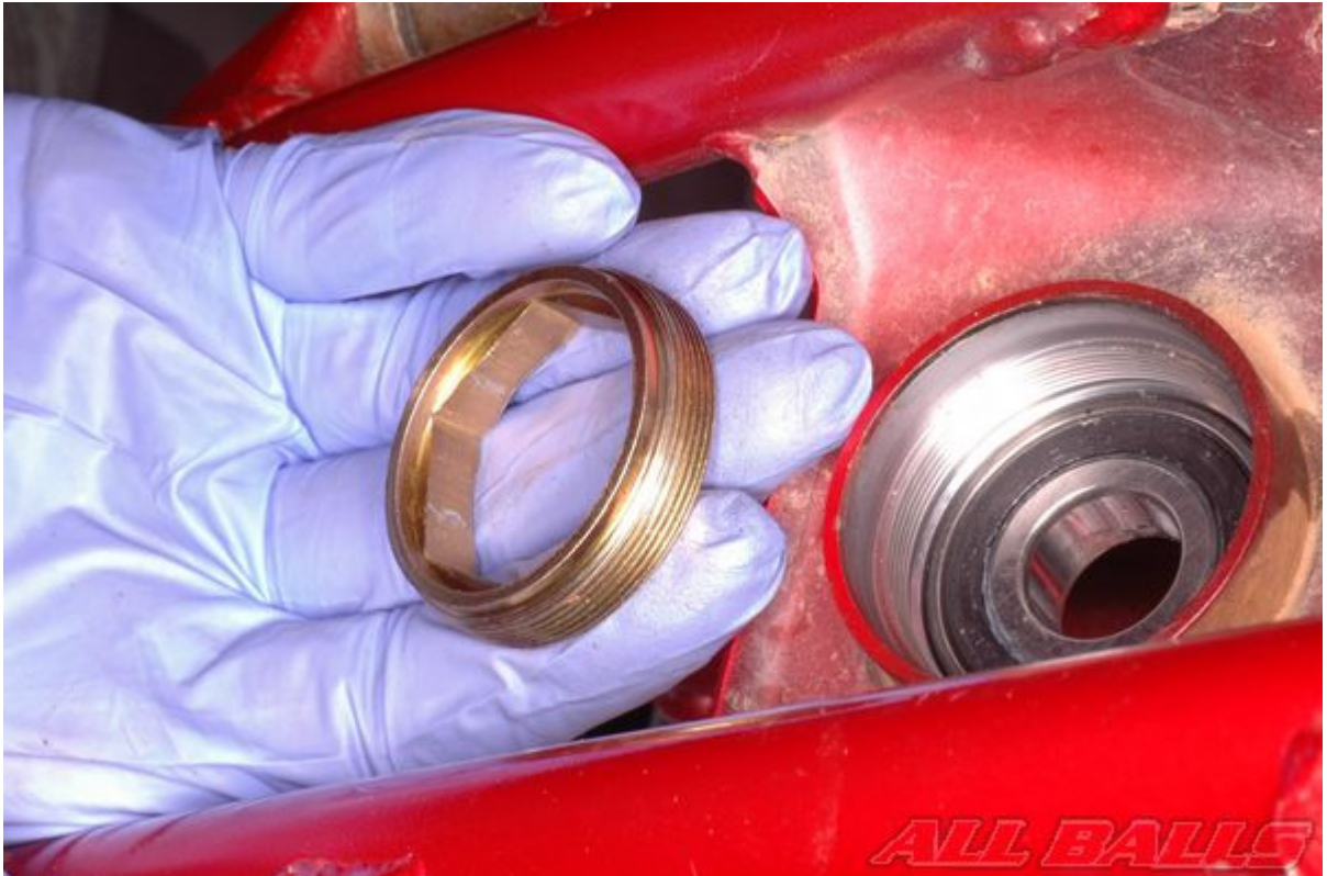
Some steering stem bearings are held in by an inner locknut. Use the appropriate special tool and remove the inner locknut.
