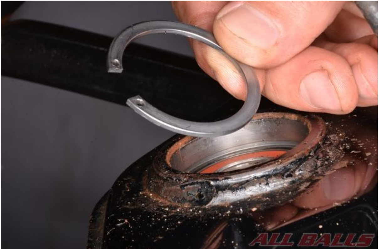
Remove the snap ring with snap ring pliers.
