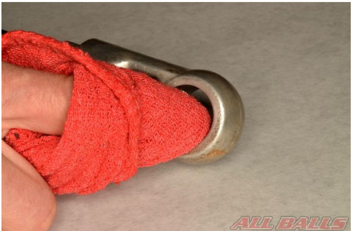
Clean away all of the old grease and rust from the bearing bore.
