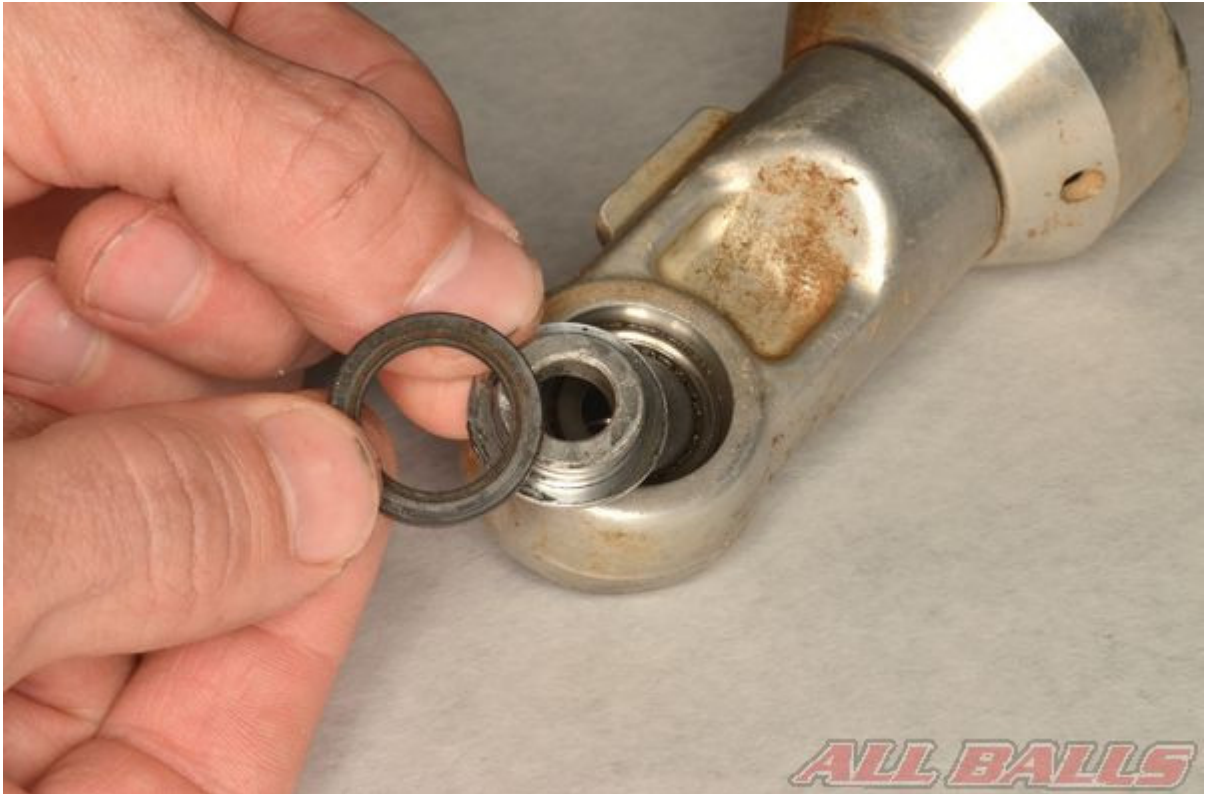
Remove the dust seals and side collars. Note the component original positions for assembly.
