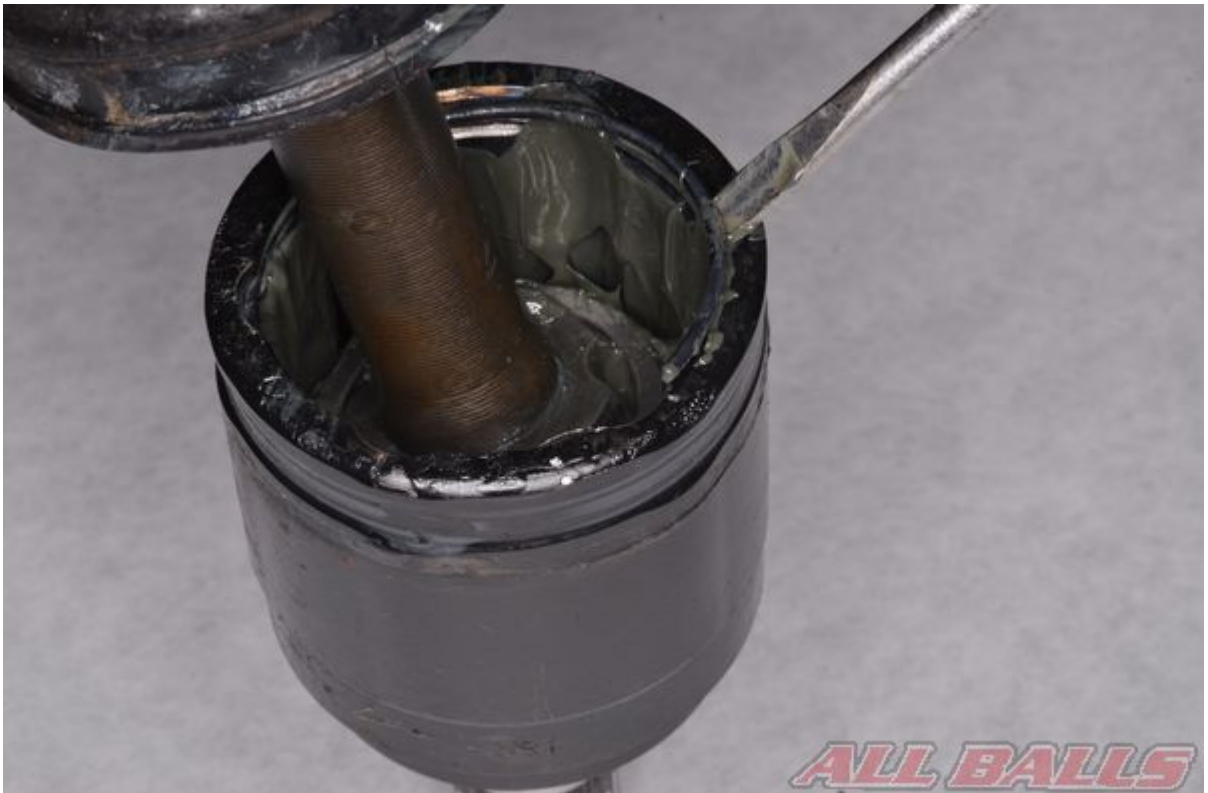
Free the plunge joint retaining ring from its groove with a small flat blade screwdriver.
