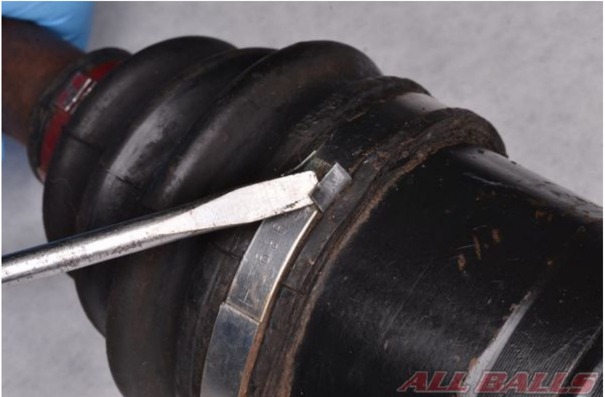
Open the old CV boot clamps.
