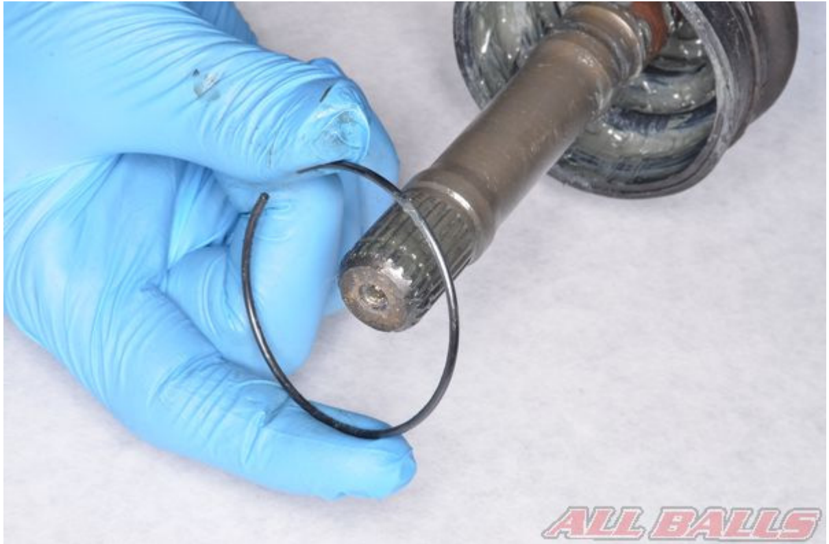
Remove the plunge joint retaining ring.
