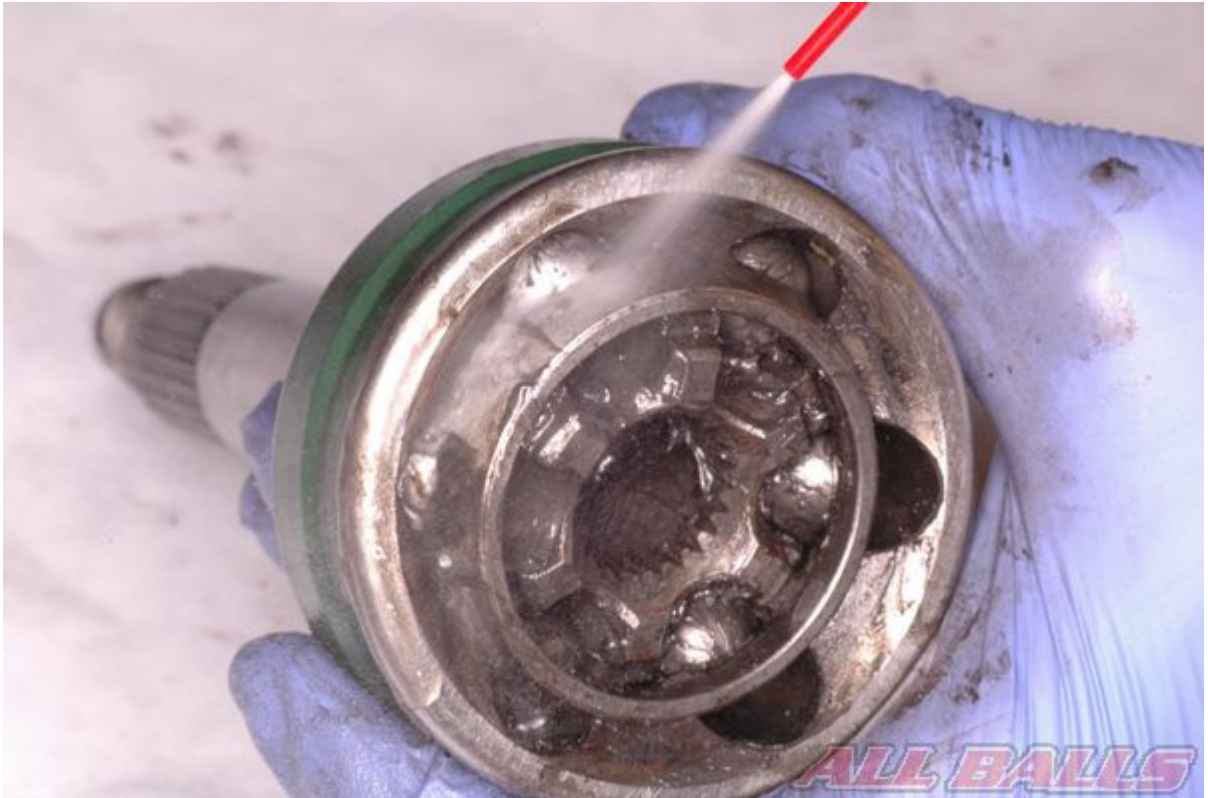
Clean out the joint to remove all of the old grease and debris.
