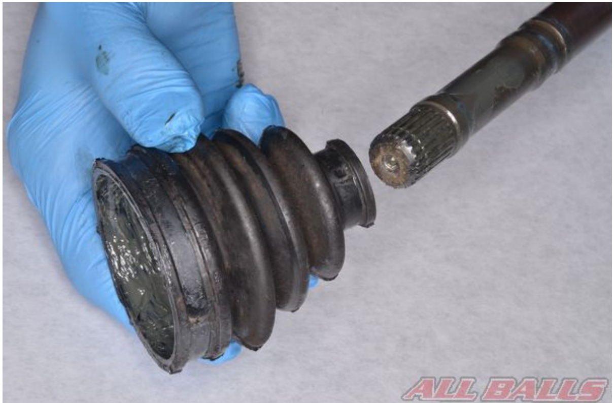
Remove the plunge joint retaining ring.
