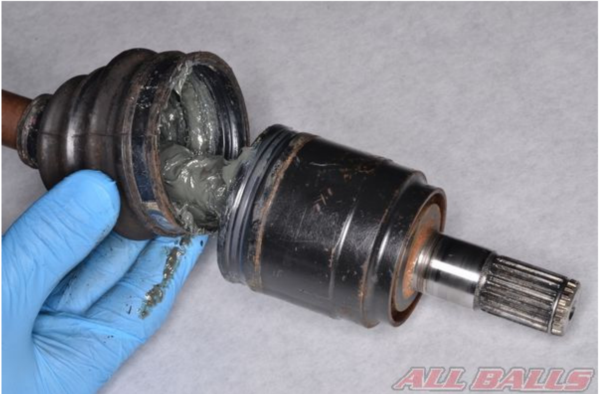
Slide back the plunge joint (inner) boot.
