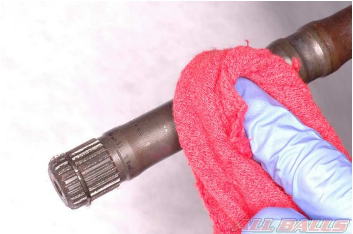
Clean the axle and inspect it for wear and damage.
