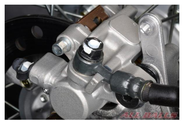
$\label{eq:make-sure-the-basis} \mbox{Make sure the brake hose is positioned correctly, and tighten the banjo bolt to specification.}$
