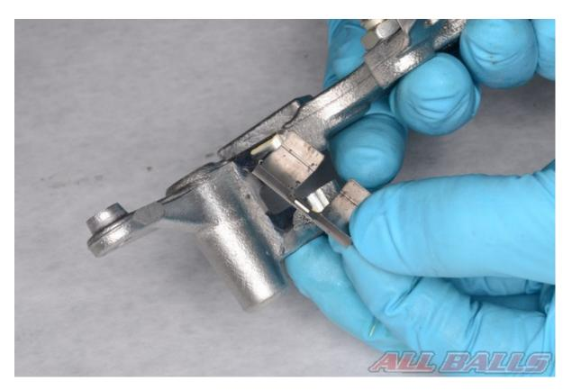
Install the brake pad retainer clip/s.
