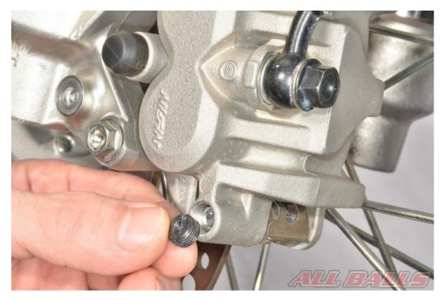
Note, some calipers may have a plug over the pad pin, have two pad pins, or not use removable pad pins at all.
