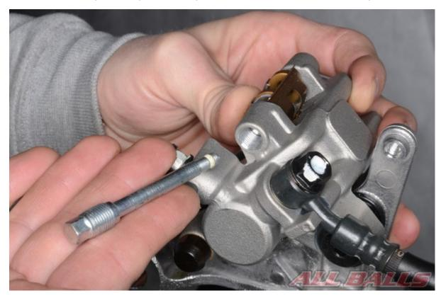
Remove the brake pad pin/s.
