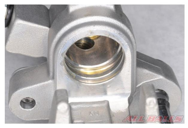
Inspect the caliper bore for damage. Measure the bore and compare to the specification.
