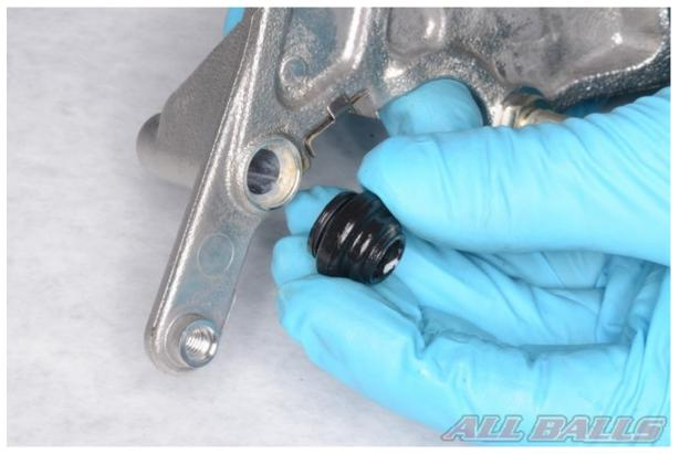
Apply a light coat of silicone grease to the inside of the slider pin boots. Install the boots.
