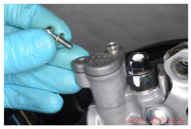
Replacement brake fluid will be needed. In most cases this will be DOT 4 fluid. The brake fluid type will often be indicated on the master cylinder reservoir cap. Always use fresh brake fluid from a newly opened container.
