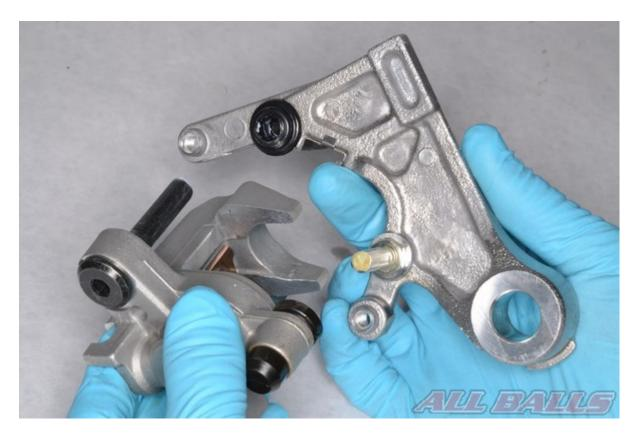
Install the caliper bracket to the caliper.
