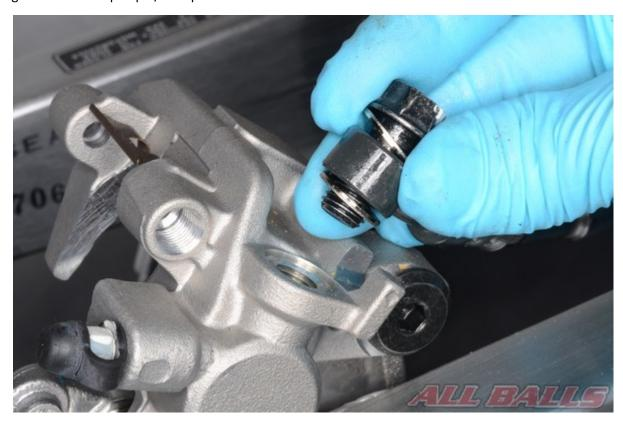
Connect the brake hose to the caliper with a banjo bolt and two new sealing washers.
