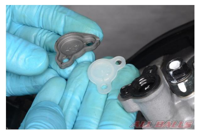
Make sure the brake fluid level is correct in the reservoir. Install the master rubber diaphragm, plastic cap and outer cap.
