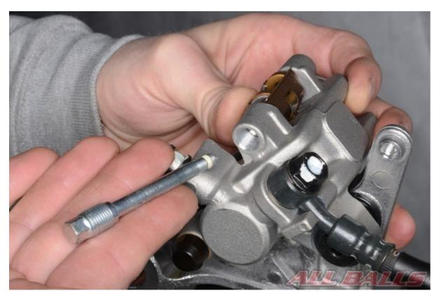
Push the pads against the pad spring and install the pad pin/s.
