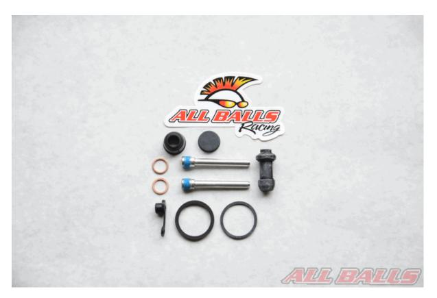
Remove the contents of your ALL BALLS RACING brake caliper rebuild kit. Layout the components in an organized manner for easy installation. Note: wait to do this until the old parts are removed and you are ready to begin installing the new components.
