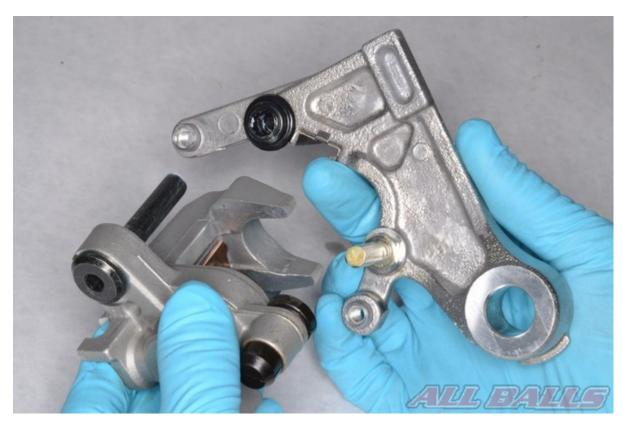
Remove the brake caliper bracket. Clean the slider pins.
