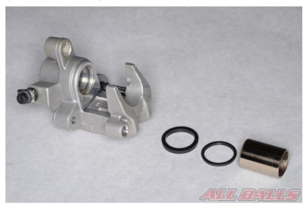
Lubricate the caliper piston/s, the caliper piston bores and the seals with the correct brake fluid from a tightly sealed container.
