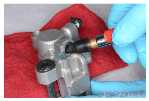
Place a 1" thick shop rag between the caliper piston and the inside surface of the brake caliper. Blow compressed air into the banjo bolt opening to remove the caliper piston.
