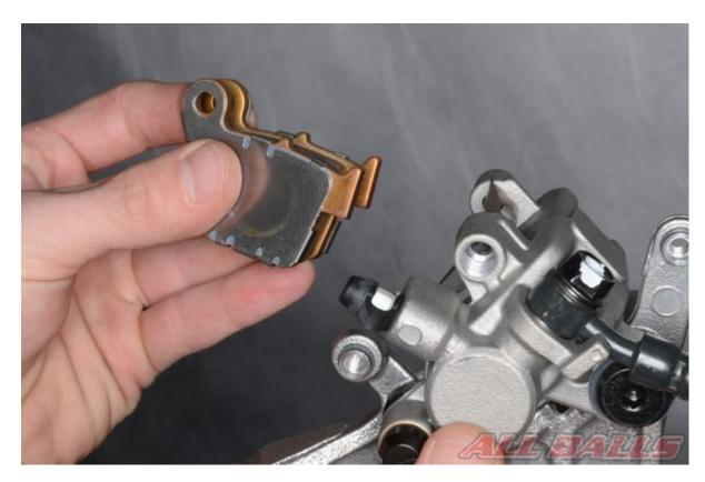
Remove the brake pads.
