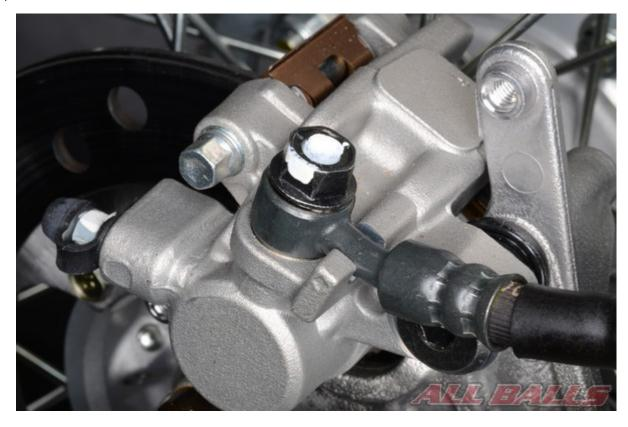
Loosen the the brake hose banjo bolt.
