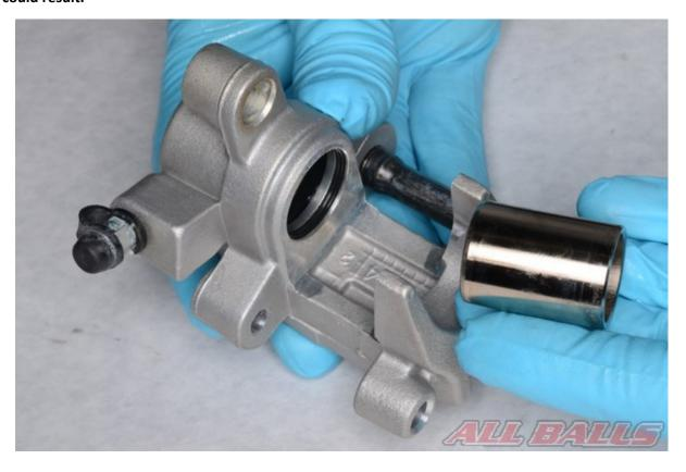
Clean the caliper, piston(s) and other metal hardware with denatured alcohol. Dry off parts with a clean rag. Inspect the caliper piston/s wear and damage. Measure the outside diameter of the caliper piston in multiple places and compare this to the specification.
