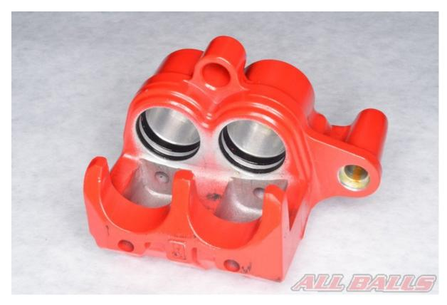
Install the new oil and dust seals. Make sure the seals are all fully seated in their grooves.
