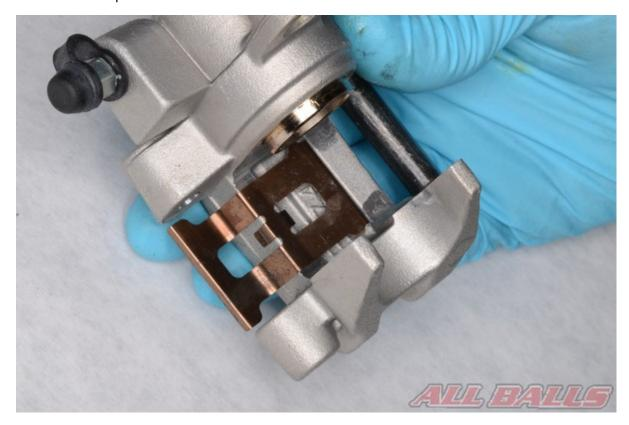
Remove the bleeder screw rubber cap.
