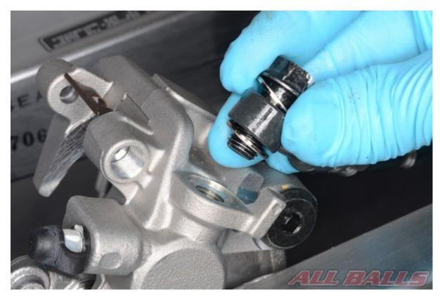
Free the banjo bolt from the caliper. Discard the two sealing washers and catch any remaining brake fluid dripping from the hose in a suitable container.
