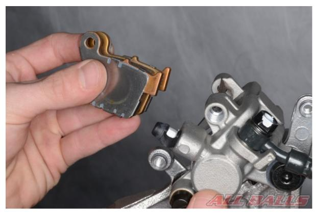
Install the brake pads making sure they remain free of any grease or contamination.
