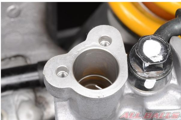
Drain the brake fluid from the master cylinder reservoir.
