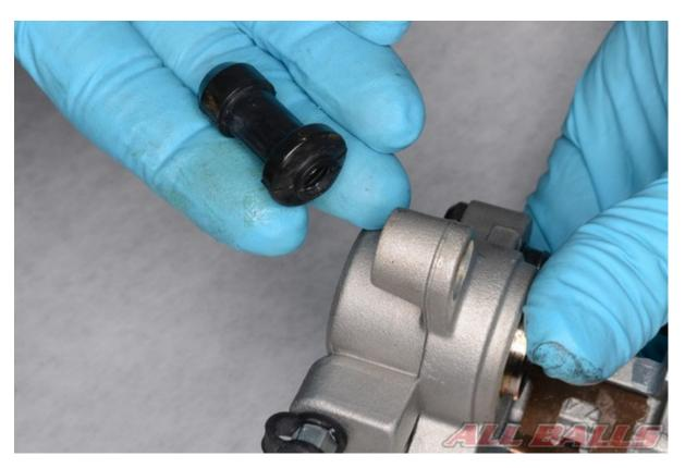
Remove the slider pin boots.
