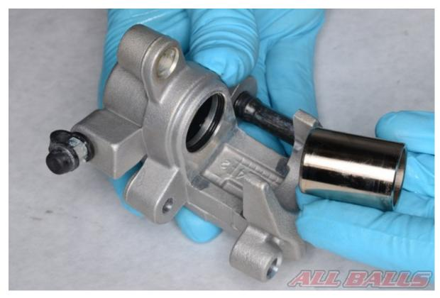
Install the caliper piston. Push the piston completely into the caliper closed end first. Use an old brake pad to push the piston all the way in.
