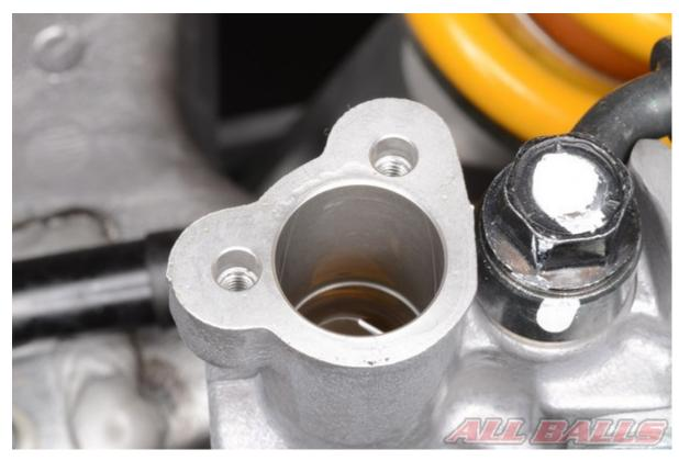
Fill the master cylinder with fresh brake fluid.
