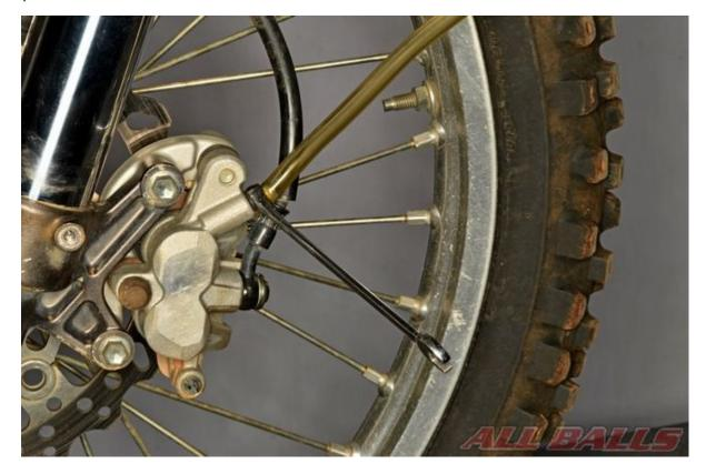
Drain the brake fluid from the system.
