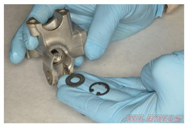
Install the washer and new snap ring.
