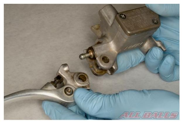
Remove the brake lever.
