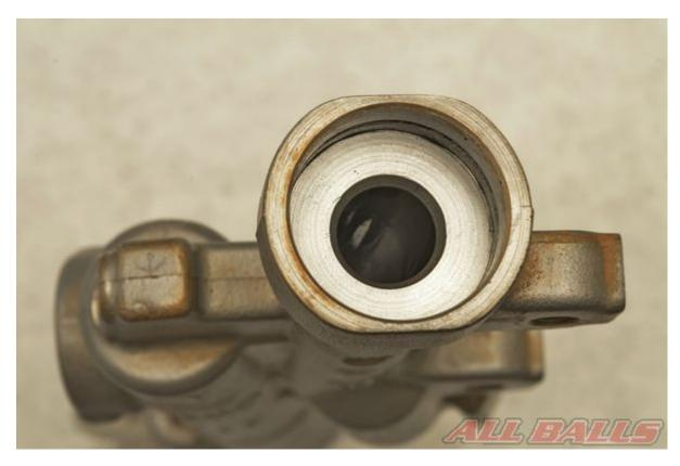
Inspect the master cylinder bore for wear and damage. Measure the inside diameter of the bore in accordance with the specification in the model's service manual. Clean the master cylinder bore and reservoir with an aerosol brake cleaner and compressed air.
