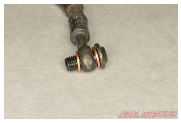
Use the two new sealing washers, one to each side of the banjo fitting. Tighten the banjo bolt to specification according to the service manual.
