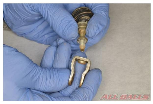
Note the position of the brake pedal height adjuster nuts. Remove the master cylinder pedal pivot.
