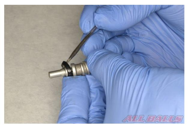
Remove the old seals from the piston, and clean the piston with an aerosol brake cleaner and compressed air.
