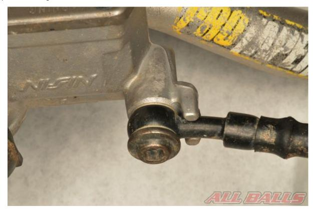
Connect the brake hose to the master cylinder.
