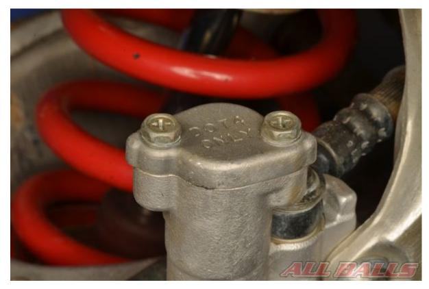
Have an unopened container of fresh brake fluid of the correct type on hand to replace the old brake fluid. Most power sports vehicles use DOT 4 brake fluid, but be sure to check the requirements for
