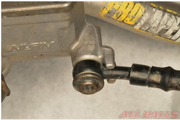
Loosen the banjo bolt and be prepared to deal with any remaining brake fluid. Free the brake hose from the master cylinder and discard the sealing washers.
