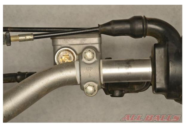
Remove the two master cylinder mounting bolts.
