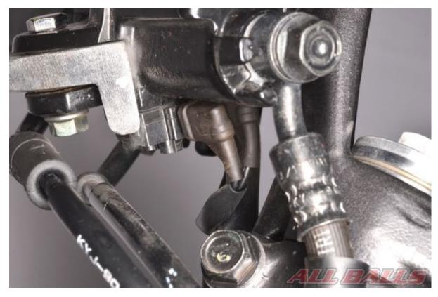
Disconnect the brake light switch if applicable.
