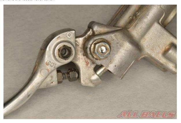
Remove the brake lever pivot nut.
