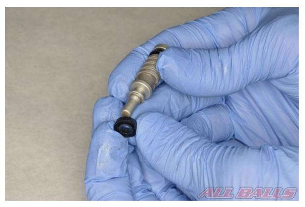
Install the new cup seals onto the piston.
