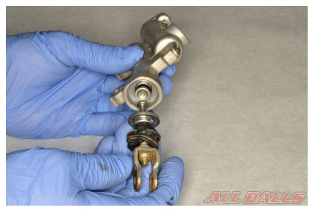
Free the snap ring from the groove with snap ring pliers. Remove the pivot rod, rubber cover, snap ring, and washer from the master cylinder.
