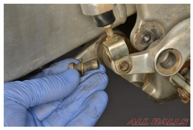
Apply a light coat of grease to the master cylinder and brake pedal pivot. Install the master cylinder pivot joint.
