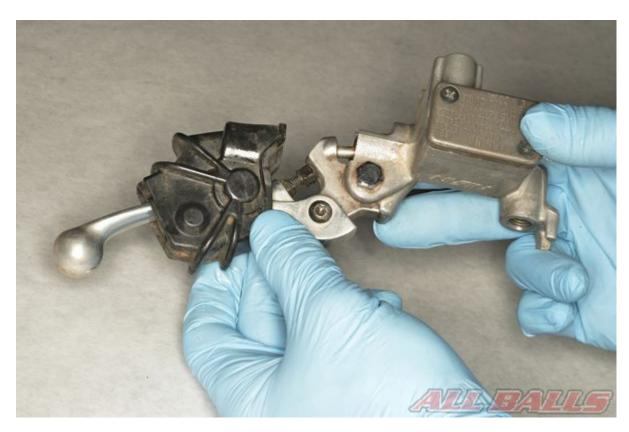
Install the brake lever rubber cover.
