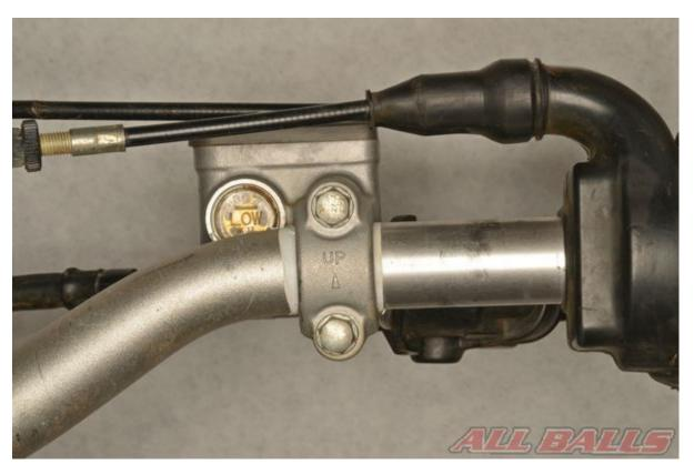
Install the master cylinder to its correct position on the handlebar. Install the perch in the correct position, and tighten the fasteners as indicated in the service manual.
