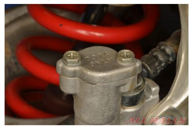
Install the reservoir cap and screws. Tighten the small screws securely while being careful to not strip them.
