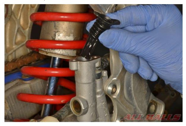
Remove the rubber diaphragm and plastic cap if applicable.
