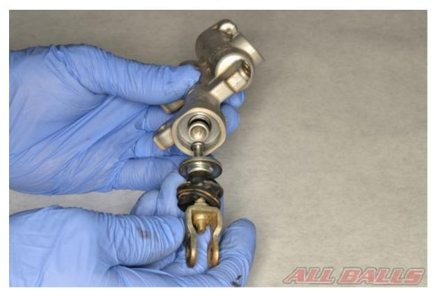
Install the pivot rod, rubber cover, snap ring, and washer into the master cylinder.
