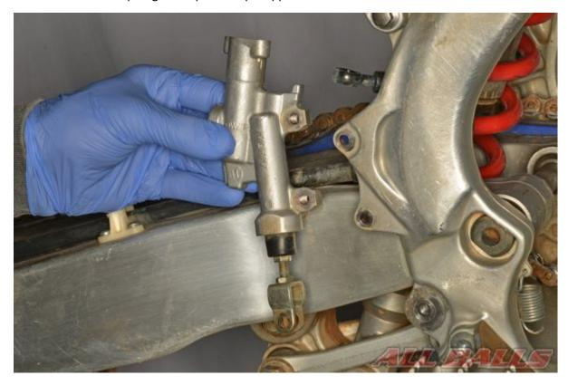
Remove the master cylinder from the frame.
