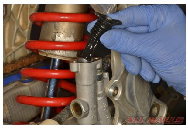
Install the rubber diaphragm and plastic cap if applicable.
