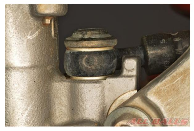
Free the master cylinder from the brake hose. Discard the sealing washers. Be prepared to deal with any remaining brake fluid that may spill when the hose is disconnected.
