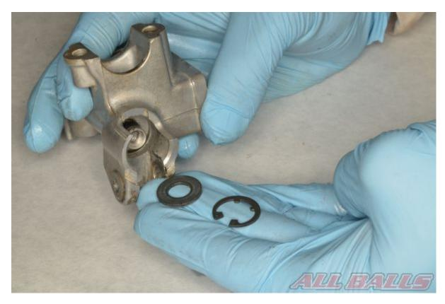
Remove the snap ring and washer.
