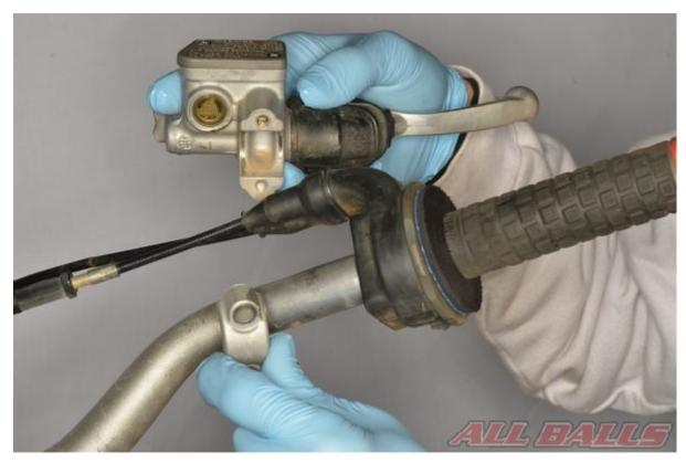
Free the master cylinder from the handlebar.
