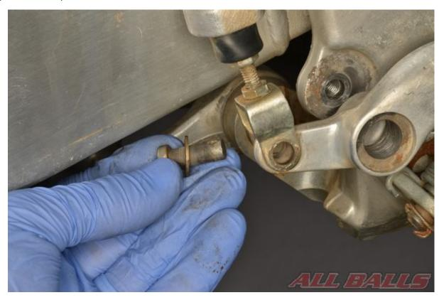
Remove the cotter pin from the master cylinder pedal pivot. Free the pivot joint from the master cylinder.
