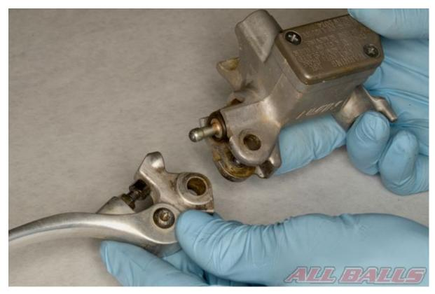
Fit the brake lever into the master cylinder.
