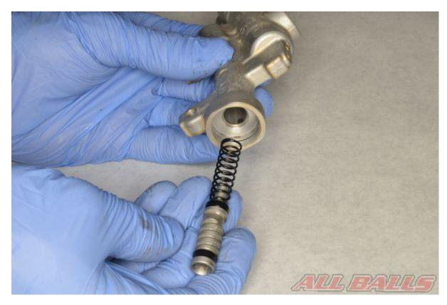
Remove the piston, seals, and spring from the master cylinder bore.
