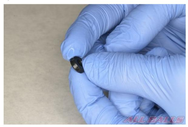
Coat the piston, seals, and bore in fresh brake fluid.
