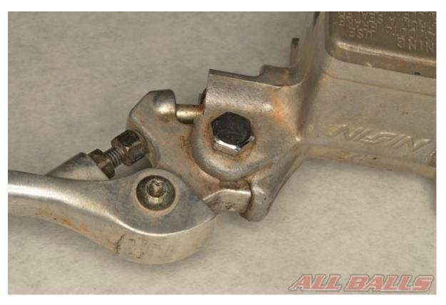
Apply a light coat of grease to the pivot section of the brake lever pivot bolt. Install the brake lever pivot bolt.
