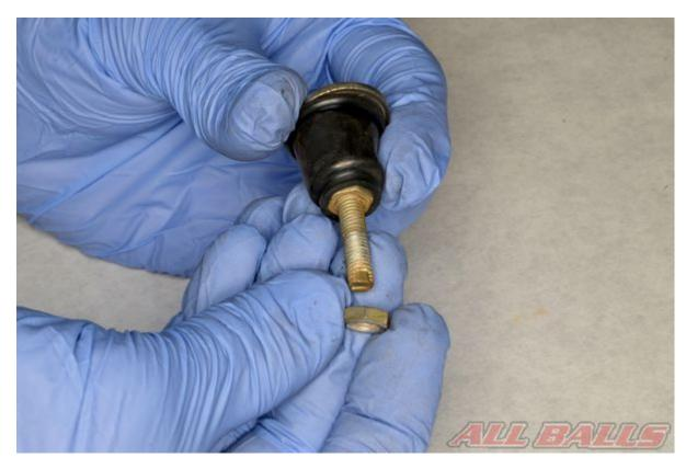
Install the the brake pedal height adjuster nuts to their original positions.
