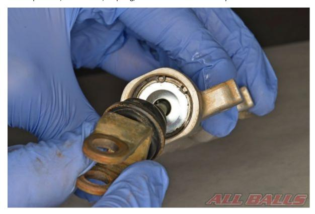
Install the snap ring into its groove with snap ring pliers. Move the rubber cover into place.
