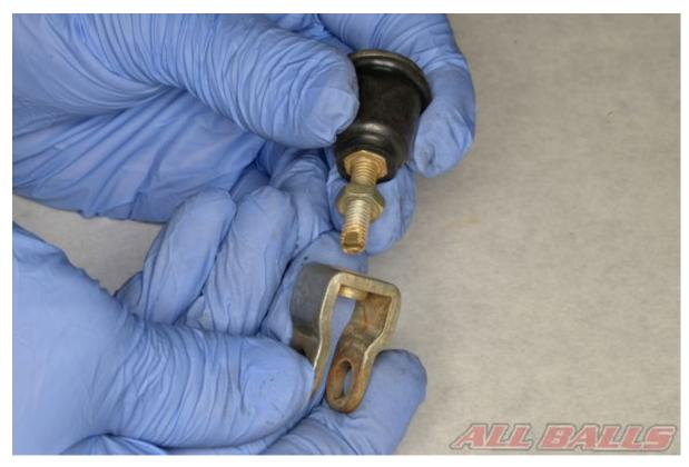
Install the master cylinder pedal pivot.
