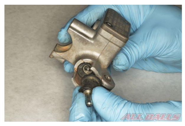
Remove the rubber cover, and lever rod if applicable.
