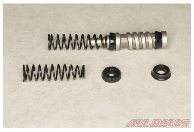
Note the position and orientation of the cup seals on the piston.
