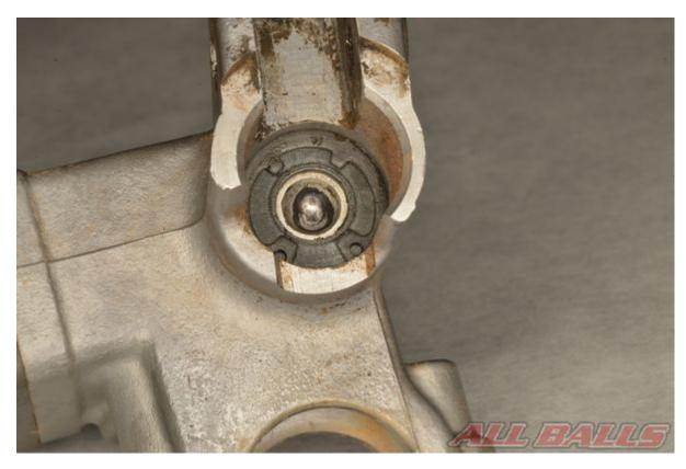
The master cylinder piston is spring loaded and held in the cylinder by a snap ring.
