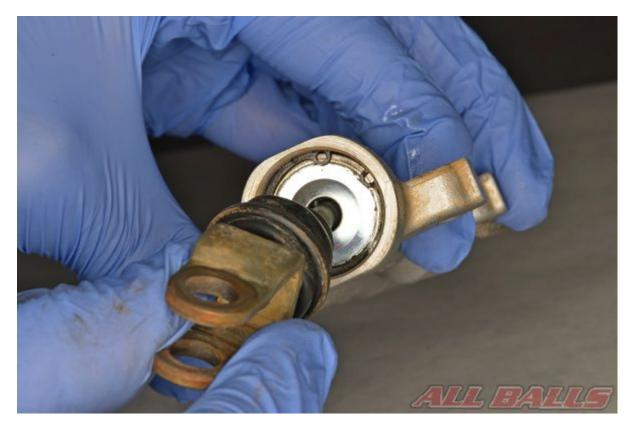
Pull down the rubber cover to access the snap ring.
