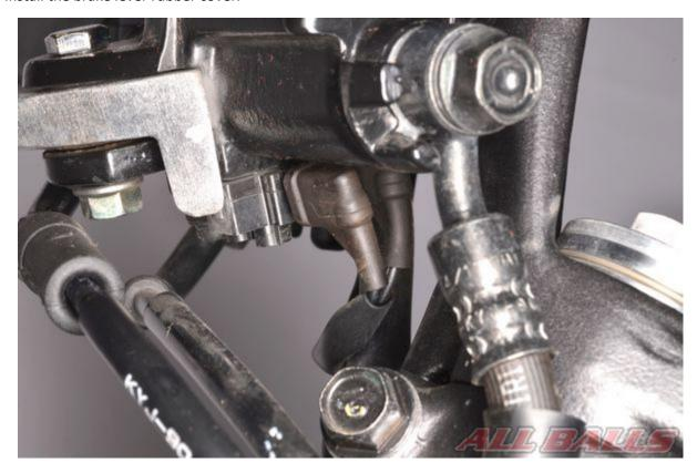
Connect the front brake light switch if applicable.
