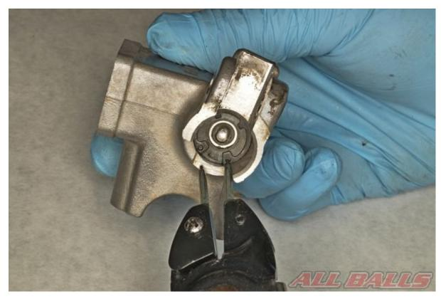
Free the snap ring from its groove with snap ring pliers.
