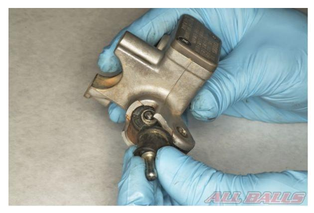
Install the rubber boot and lever rod if applicable.
