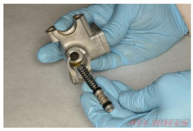
Install the spring and piston into the bore together.
