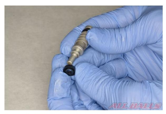
Install the new cup seals onto the piston.
