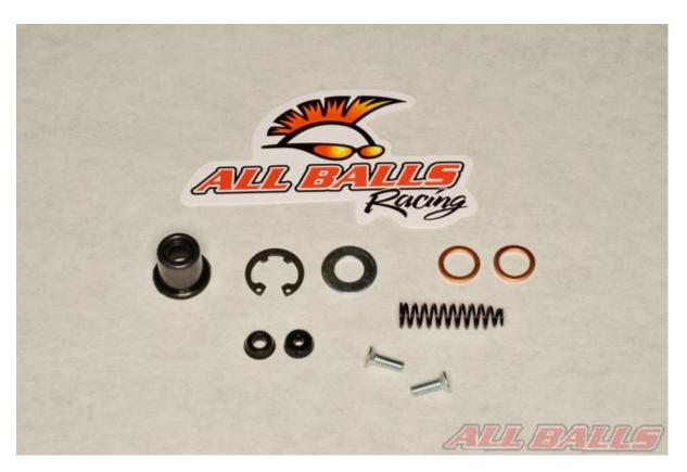
Remove the contents of your ALL BALLS RACING master cylinder rebuild kit. Layout the components in an organized manner for easy installation. Note: wait to do this until the old parts are removed and you are ready to begin installing the new components.
