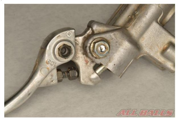
Install the brake lever pivot nut.
