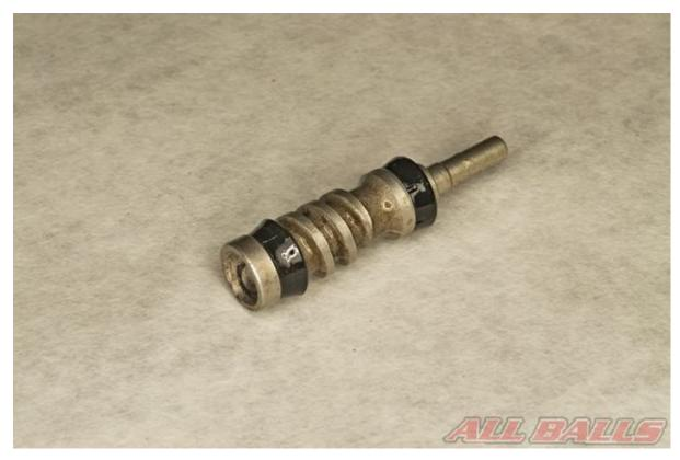
Inspect the piston for wear and damage. Measure the outside diameter of the piston in accordance with the specification in the model's service manual.
