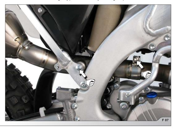
4. Align the muffler in respect to the motorcycle and tighten the muffler's bracket bolt (using stock bolt and washer from Akrapovič installation kit), link pipe's bracket bolt and clamp to the specified torques (F 08, 09).
