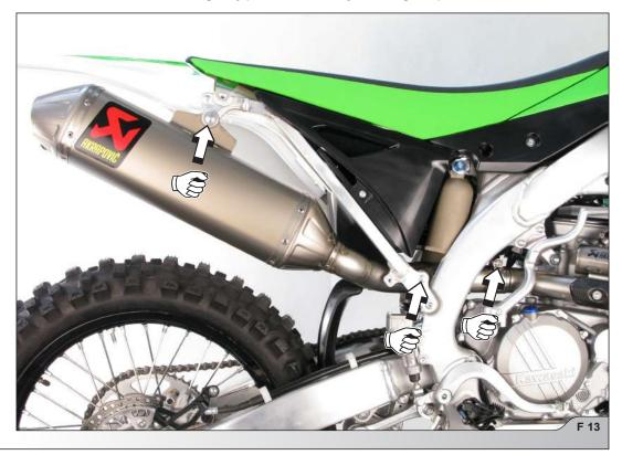
8. Align the muffler in respect to the motorcycle and tighten the muffler's bracket bolt, link pipe's bracket bolt and clamp to the specified torques (F 14, 15).
