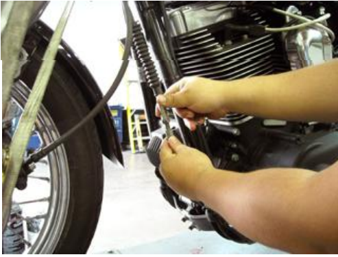
13. Adjust the clutch cable. Ensure free play of 1/8" or more at the clutch lever pivot between the clutch holder and lever without pulling the cable.
