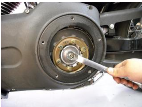
3. Loosen lock nut on the clutch adjuster screw.
