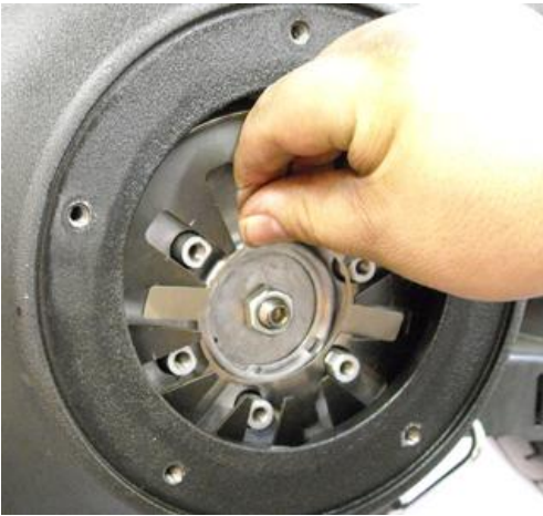
9. Install base plate. Starting with widest tab on the base plate insert it inside the diaphragm spring.
