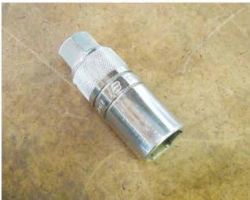
Tech Note: You can use 18 mm spark plug socket to tighten lock nu t.
