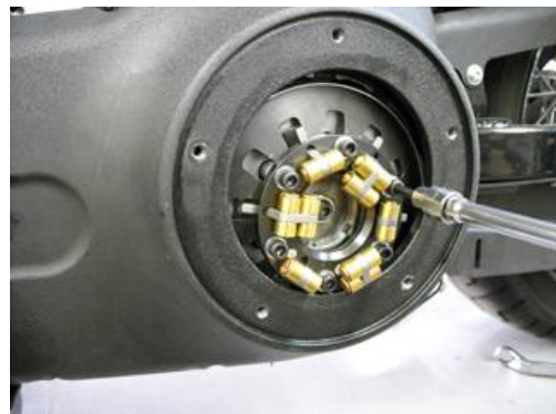
12. Use the provided bolts and tighten evenly with a 5 mm Allen wrench. Ensure the diaphragm spring is not out of position and start tightening the bolts. Finally, tighten to a torque of 90-110 in-lbs (10.2-12.4 Nm).
