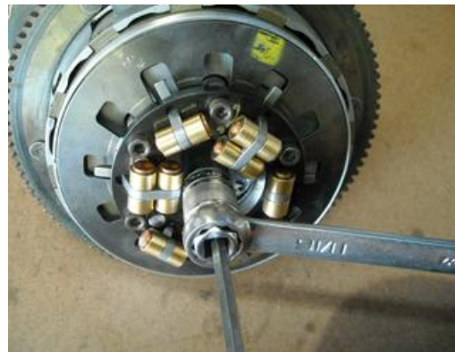
Tech Note: Adjusting adjuster screw with using 18 mm spark plug socket.
