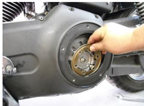
6. Pull the spring retainer and remove it.
