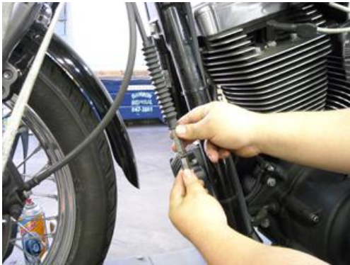
1. Turn cable adjuster until there is a large amount of free play at the clutch hand lever.
