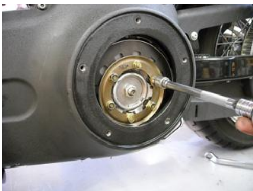
5. Loosen the spring retainer evenly a little at a time using a 10 mm socket wrench.
