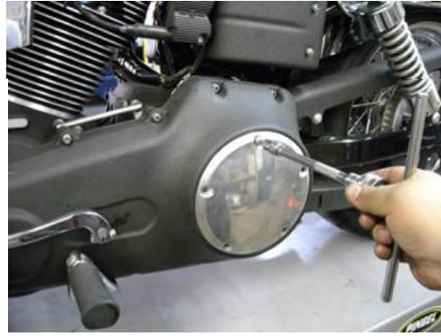
14. Install derby cover gasket (Parts#AIM003-001) and derby cover. Tighten bolts to 84-108in-lbs (9.5-12.2 Nm).
