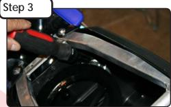
Using a 4mm allen wrench, loosen the clamp around the air boot flange.
