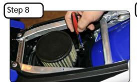
Using a 1/4" socket and ratchet, tighten the hose clamp on the inner Pro GUARD 7 filter.
