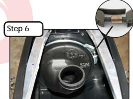
Tighten the clamp using the 4mm allen wrench. You may have to remove the spacer in the clamp to completely tighten.
