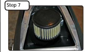
Install the inner Pro GUARD 7 filter onto the intake tube.
