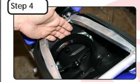
Carefully pry the plastic foam air filter mount out of the air boot flange. You should be able to remove the mount with your fingers.
