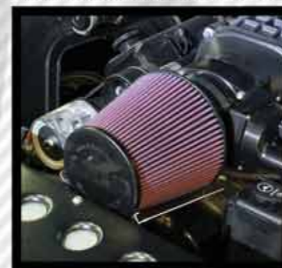
Built-in provision to mount an IAT (Intake Air Temperature) sensor
