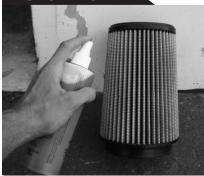
You can wash your Pro Dry S filter and return it to 100% of its original airflow. Remove the filter from the intake kit and simply spray the filter with .aFe cleaner and let sit for 10 minutes.
