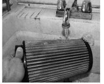
Rinse the filter with clean water to remove the dirt and excess cleaner. Continue rinsing until the water runs clear.
