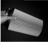
You can tap your Pro Dry S filter and return it to 85% of its original airflow. Simply remove the filter from the intake kit and lightly tap it on a solid surface. Tap and turn the top and bottom of the filter until most of the visible dirt has been released. Reinstall the filter in your vehicle. Do not apply oil to the filter.
