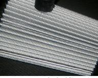
You can vacuum your Pro Dry S filter and return it to 96% of its original airflow. Remove the filter from the intake kit and vacuum away the dirt using a shop vacuum or regular house vacuum. Reinstall the filter in your vehicle. Do not apply oil to the filter.
