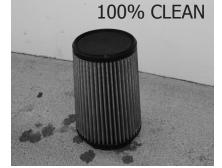
Allow the filter to dry completely (our synthetic media dries quickly and should dry within a few hours in normal conditions). Reinstall the filter in your vehicle. Do not apply oil to the filter.
