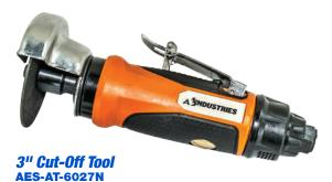
Holds 3" cut-off wheels with a 3/8" arbor hole. Features a built-in 4 position air regulator with preset RPM speeds. Excellent for cutting sheet metal, tail pipes, bolts and nuts.
