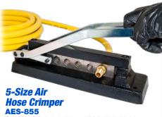
Can crimp 1/4" single braid up to 3/8" double braid air hose. Five popular die sizes are instantly available and it's simple to operate. Self-contained, no separate dies to lose or misplace. The dies are ribbed and made from hardened steel. Can be permanently mounted or used portably.
