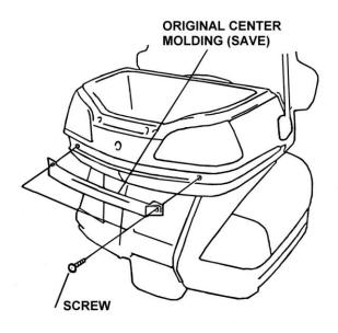
4. Install the right, left and center moldings from the kit on the trunk in the reverse order of removal.
