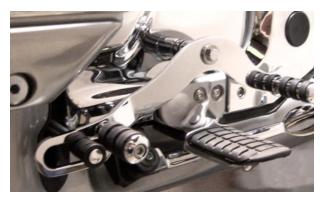
**4.** With the longer bolts supplied, sandwich the Heel Toe Shifter plate between the frame and chrome bracket provided.
