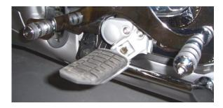
3. Install shifter slot over shifter peg.
