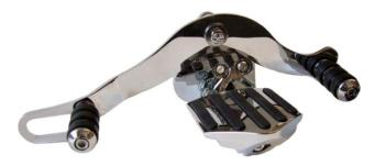
**8.** Right side. Remove stock bracket and peg. Replace with chrome bracket and floorboard with stock bolts.
