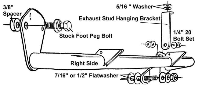
6. Remove the stock shifter rubber and cut off the two inside rings. (This makes room for the heel-toe shifter fork.) Mount the left hand floorboard support by sliding the shifter fork onto the clear area on the stock shift pedal. Secure the rear mount to the stock foot peg using the ½" spacer, one 7/16" flat washer and the stock lock washer and acorn nut. Leave loose.
