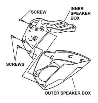
**9.** Locate a mark on the left speaker box and drill a hole thru the mark using an electric drill motor, starting with a 3 mm, 6 mm and 10 mm drill bit. Remove any burrs from the edge of the hole.
