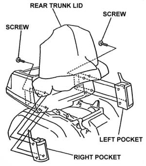
5. Remove the 13 screws and the inner lid from the trunk lid as described in the Service Manual.
