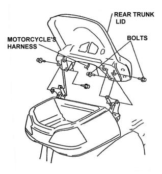
**7.** Remove the bolts, screws and the right and left speaker boxes from the trunk lid.
