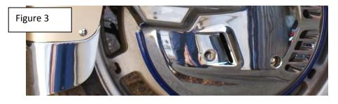
5. Put on the new rotor cover using the original bolts. Replace in reverse order.
