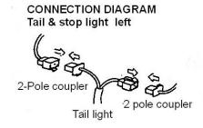
**2.** Disconnect the left side tail light/stop light connectors and connect the plugs from the new center light in series as shown.
