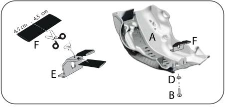
1 - Insert the included bolts (B) and the bushings (C) into the Acerbis Skidplate as indicated in the image.
