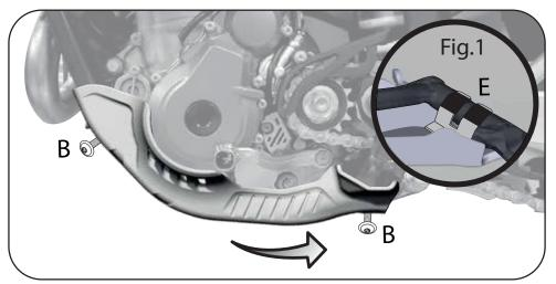
3 - Position the Skidplate so that the bracket (F) is positioned over the frame rail (Picture 1). Secure the front of the skidplate up against the frame rails and tighten the 2 bolts (B). Lastly, secure the back of the Skidplate to the frame by tightening the bolt (B) in the bracket (E).
