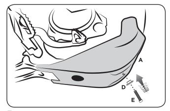
5. Secure the skid plate to the previously installed bracket, using the socket and screw supplied.
