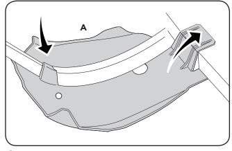
**4** Ensure that the clips of the skid plate are properly inserted on the frame.
