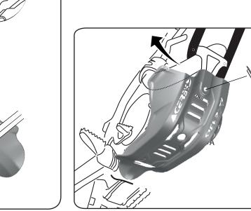
**3.** Screw the skid plate to the frame.
