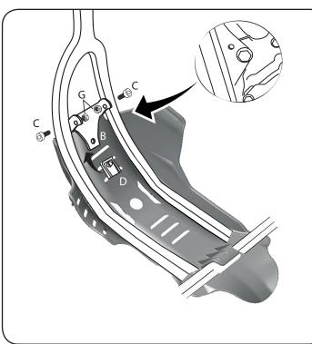
2. Assemble the clip on the clamp and place the clamp on the frame as indicated.
