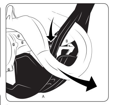
1. Disconnect the exhaust pipe and move it forward to facilitate the mounting of the clamp to the frame.
