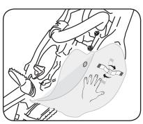
5. Push the skid plate and screw 90° the bracket
