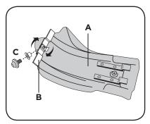
2. Screw two turns the screw on the bracket
